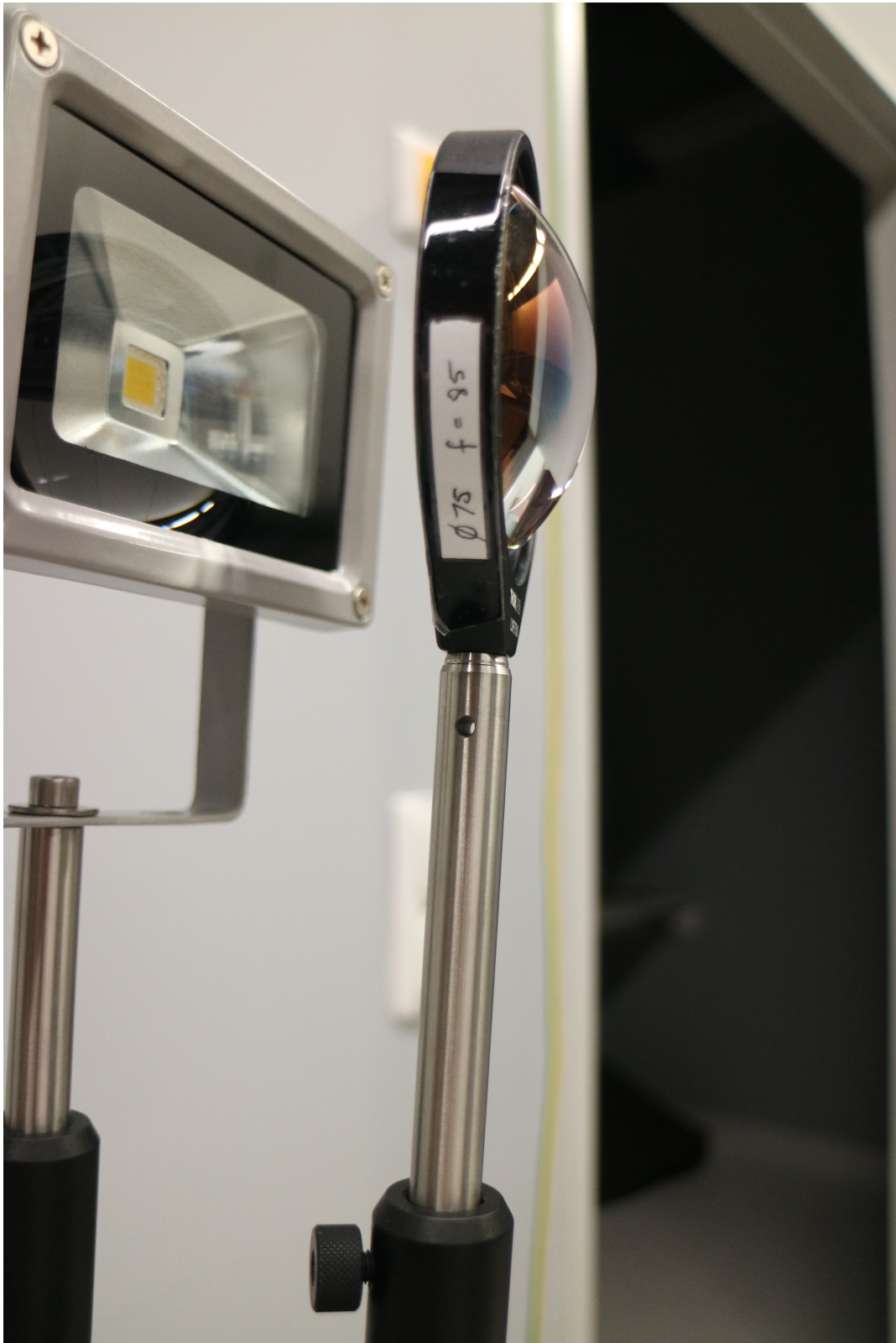
Figure 3.18.: 10-Watt LED lamp with beam-expanding lens. Used as backlighting for Lagrangian Particle Tracking.
