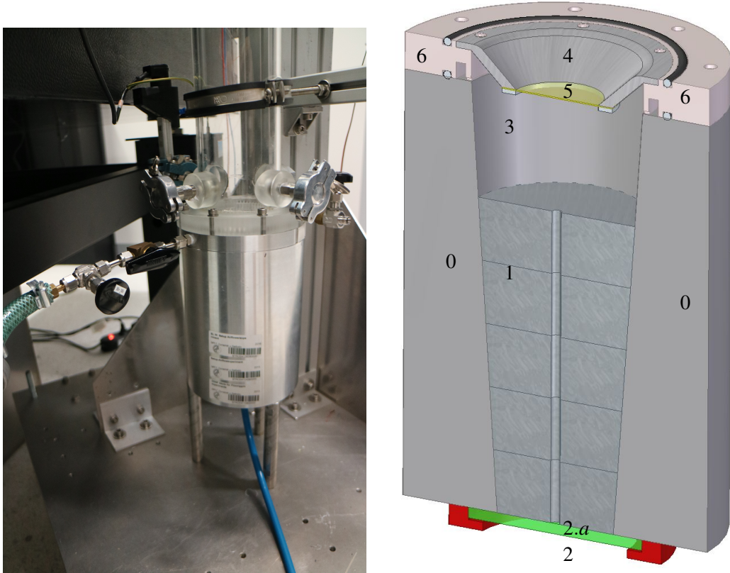
Figure 3.4.: Photograph (left) and cut-away view of the apparatus base. (0) The external holder is solid aluminum. (1) The interior is a cone of stacked sintered-metal cylinders of porosity coefficient \chi . (2) The air inlet is at the bottom. Shown is a dust filter (2.a), although there is also the option to attach an adaptor that delivers pressurized gas to the inlet (see blue tubing in photograph). (3) The hollow chamber provides the option to add additional flow-impeding material. (4,5) The tray installed above the chamber is the particle-seeding bed; (4) The tapered part of the tray is made of aluminum and (5) the flat bottom is a fine wire mesh through which air can pass, but solid particles cannot. (6) Also shown is the perforated ring, through which gas can be injected directly into the system, without passing through the metallic filter (see valve assembly in photograph and details in figure 3.5).
