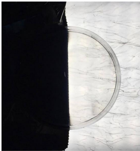
Figure 8. Darth Vader assay arena. A Petri dish with agar is placed on an acrylic pane with white light LED's. Half of the dish is painted black and covered with aluminium foil. A larva is placed in the middle and allowed to choose between dark and light.
