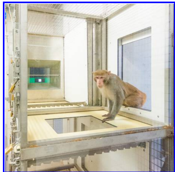
Fig. A1. XBI inside a housing environment. The XBI replaces a wall of a single cage compartment (back, displays a task not used in this study). An opening connects those compartments to the housing cage of the social group (right). During a training session, the animal was isolated in the compartment with the XBI attached.
