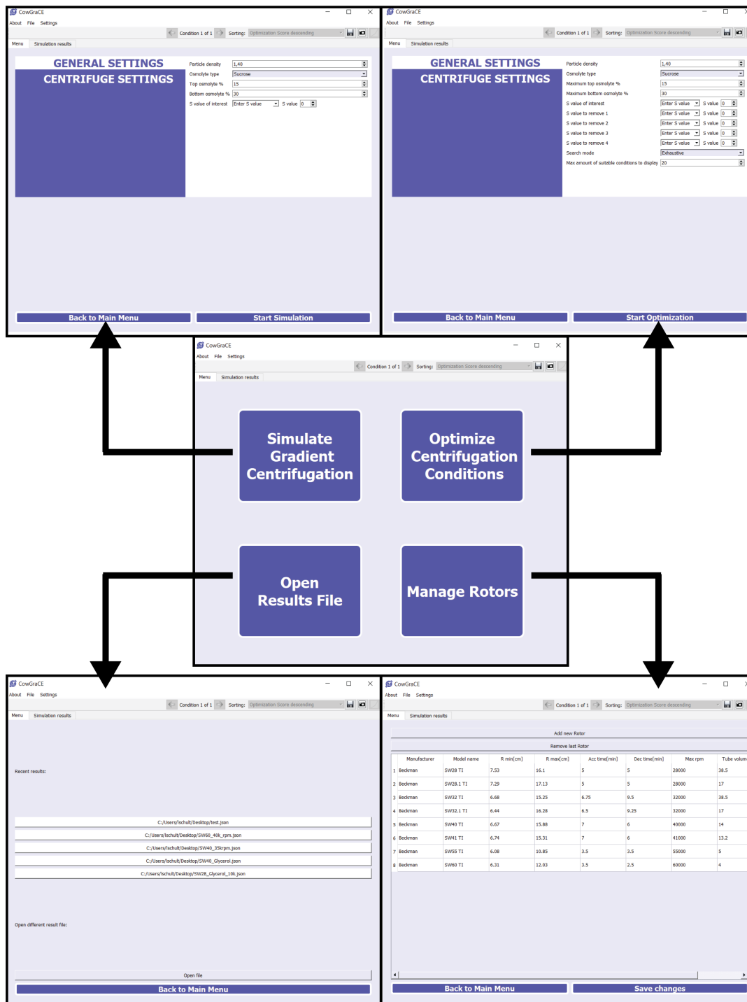
FIGURE 3.16: CowGraCE main window. Shown in the middle is the main menu from which the result loading widget (bottom left), the rotor management widget (bottom right) and the simulation and optimization modes (top left and top right) can be started.
