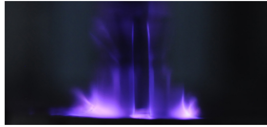
Figure 4. Coplanar surface barrier discharge (CSBD), exposure time: 1/3 s.
