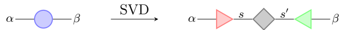
Figure 4.3: Pictorial representation of the singular value decomposition of a matrix M \in \mathbb{C}^{m \times n} into U \cdot \Sigma \cdot V . The result consists of a right orthonormal tensor (red triangle), a diagonal matrix (grey diamond), and a left orthonormal tensor (green triangle).
