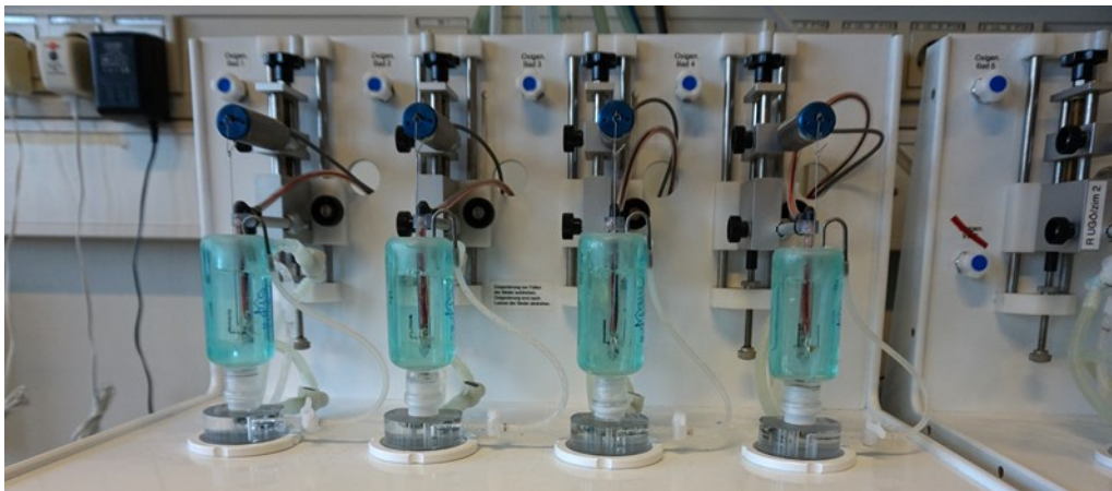
Figure A 6 Organ bath apparatus for isometric force measurements
