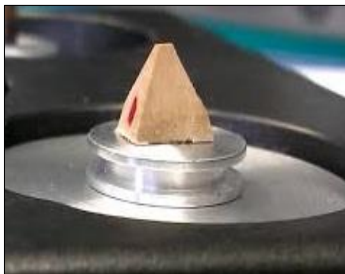
Figure 7.1: Cropped pyramid shape sample for SEM analysis before modification.
