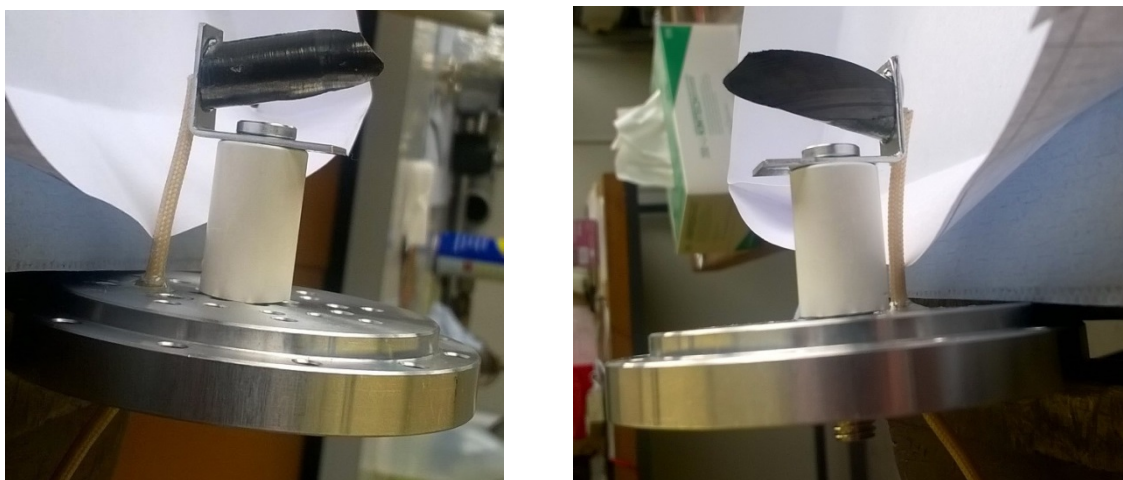
Figure 5-3: Picture of the CuO single crystal mounted to a sample holder on the bottom lid of the sample can. The beige wire belongs to a Pt100-thermometer which is glued as close to the sample as possible.
