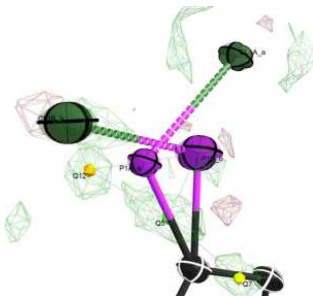
Figure 8.5: Difference electron density after refinement with disordered PCI-groups at the 0.082 eÅ -3 level.
