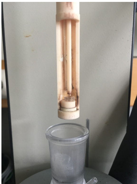
Fig. 3: Sample holder as used for viscosity determination by using the micropenetration technique.
