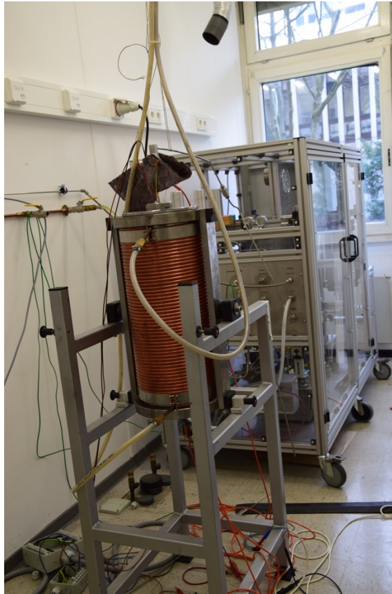
Fig. 6: Internally Heated Pressure Vessel (IHPV).
