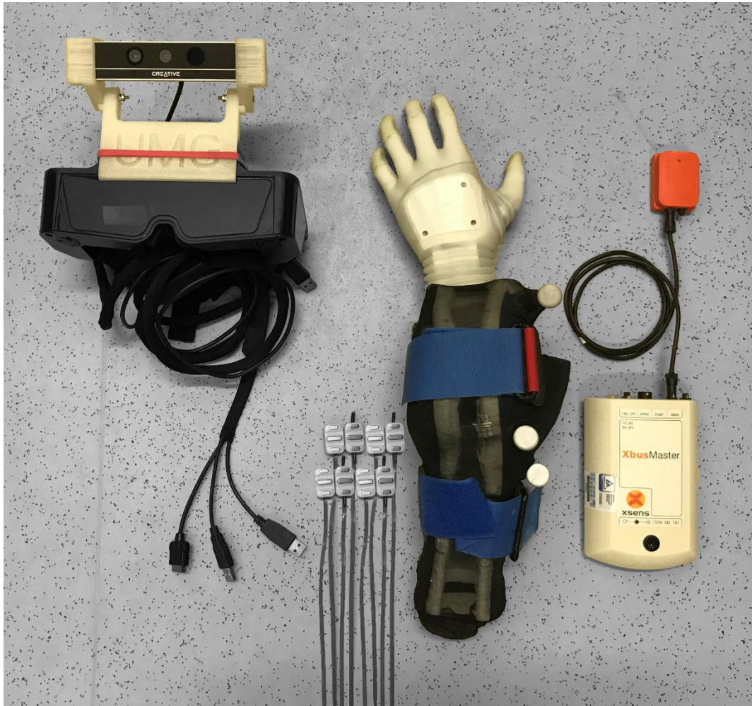
Figure 2.1 Photography of the material used with highlight of the components used for the artificial proprioception module. Those were the RGB-D camera, the sensors embedded in the prosthesis, the IR Markers placed on the socket, and the IMU fixed on the socket.
