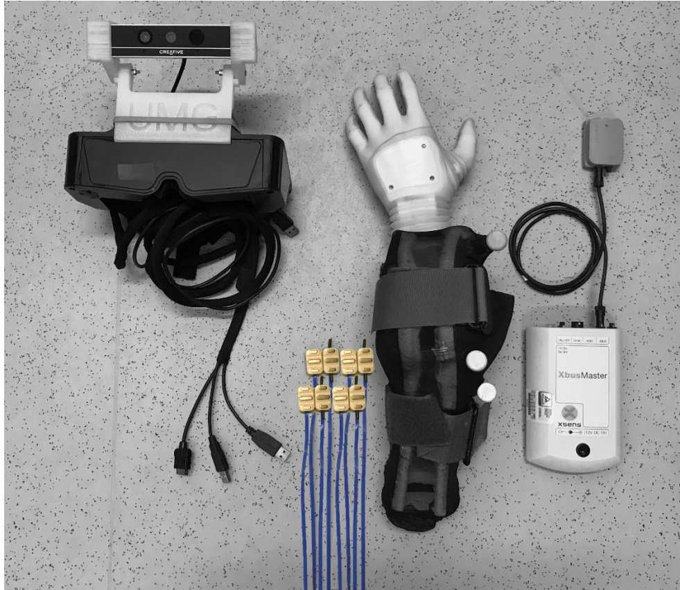
Figure 3.1 Photography of the material used during the experiment with the highlight of the electrodes. Eight DC electrodes were used to acquire the EMG signals around the forearm of the participant.
