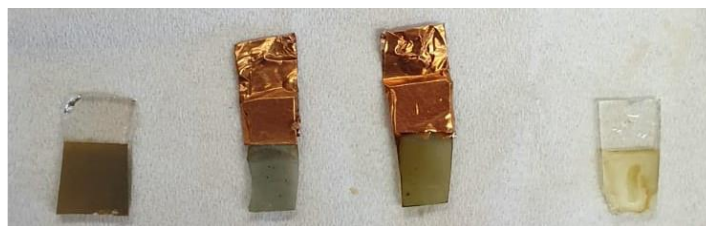
Figure 4.18. Representation of the ITO| meso ITO| 4 electrodes before, after immersion in aqueous HOTf (0.1 M, pH = 1), immersion in an aqueous phosphate buffer (pH = 7), and after rinsing with methanol to remove the nonimmobilized species (from left to right).
