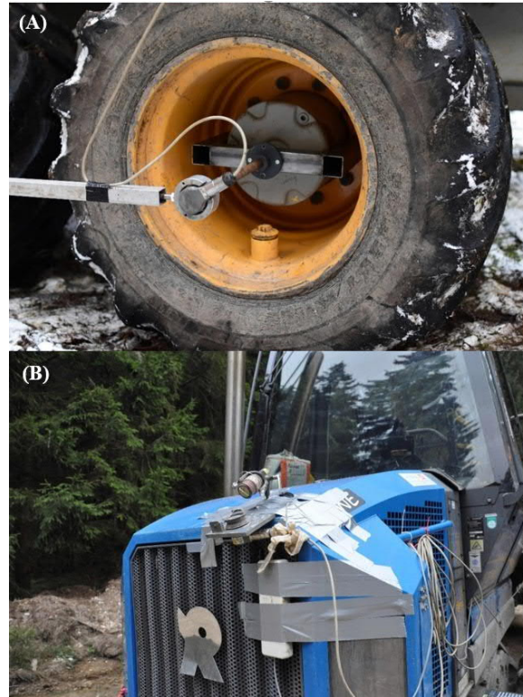
Figure 6-3. Installed incremental rotary encoder sensor to measure wheel speed, mounted on the second wheel of the front bogie-axle (A) and on the front part of the machine for capturing travel speed (B).
