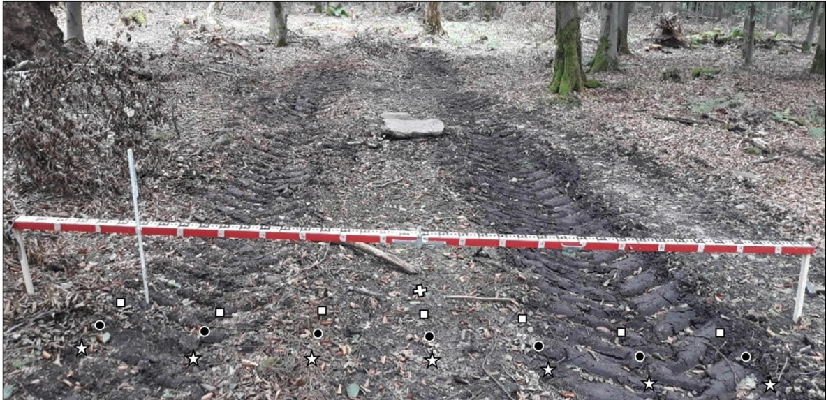
Figure 2-2. Example of a cross-sectional measuring transect on a machine operating trail. In-situ measurements were performed in advance of the regularly planned CTL thinning operation, using a Penetrologger (squares), vane tester (circles), a dual-mass dynamic cone penetrometer (cross) and a TDR probe (asterisks) as described in section 2.2.3 . The levelled reference beam, positioned on wooden pegs and a yardstick were used to determine rut depth ( Figure 2-3 ), as it occurred during the given operation.
