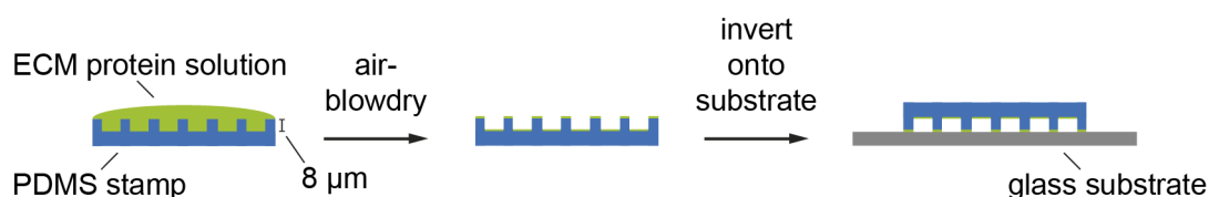
Figure 2-7: PDMS stamping on glass substrates. 8 \mu\text{m} deep PDMS stamps were incubated with 20 \mu\text{g}/\text{ml} of Synthemax ® for 30 minutes. The protein solution was then air-blowdried off, and the stamps were inverted onto the glass substrates, which had priorly been rendered hydrophilic using a plasma cleaner. Finally, the stamps were removed and the substrates were incubated with a 0.1 mg/ml solution of PLL-g-PEG to block unstamped regions.
