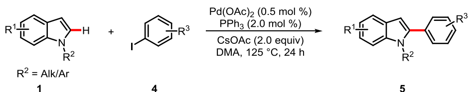
Scheme 6: C2-selective C–H arylation of N -substituted indoles 1 .
