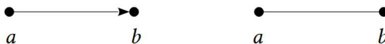
Figure 3.2.: A directed (left) and an undirected graph (right), containing two vertices a and b , as well as one edge.
