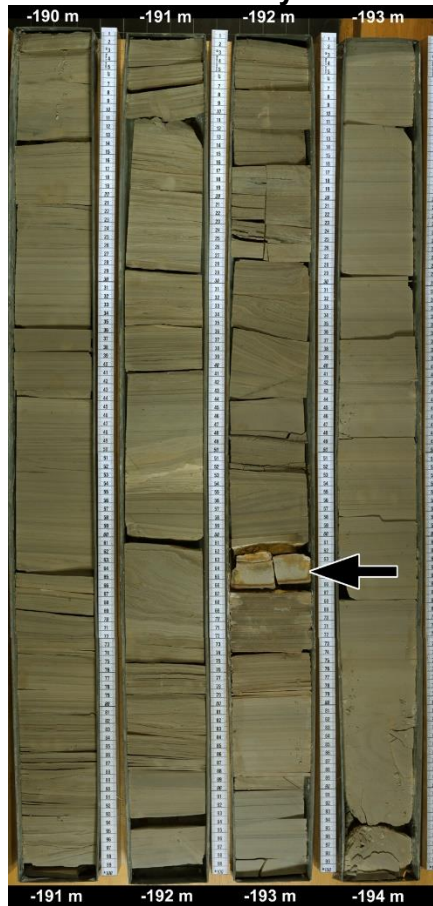
Figure 3.4 Volcanic-ash derived buddingingtonite bed (arrow) in the laminite member at 192.61-192.66 m core depth, drilling NR 1003.
