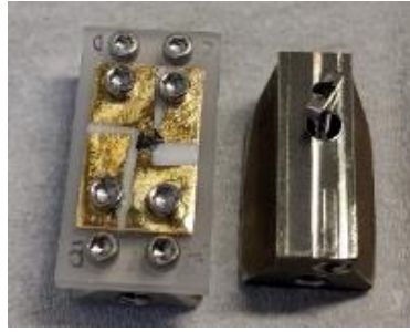
Figure 5.6 Cleaved \text{Na}_2\text{IrO}_3 sample for transport measurements. On the left, the contacted sample mounted on the holder for transport measurements is seen. On the right, the hole-base with cleaver and second half of the sample is visible.
