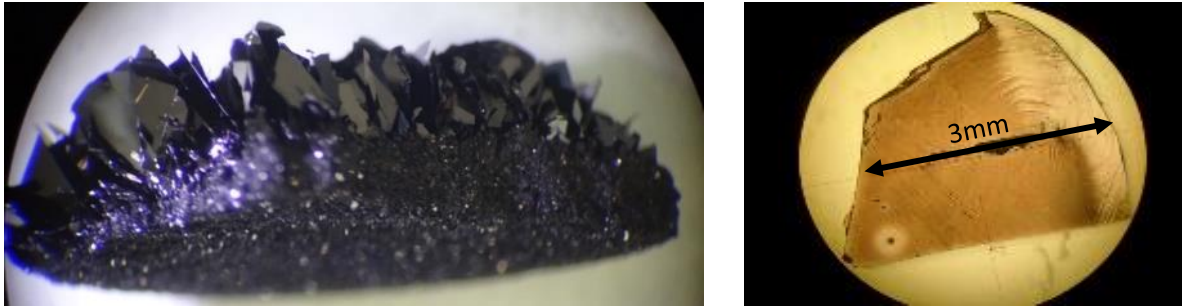
Figure 5.1: Plate shaped sodium iridate crystals grown out of \text{Na}_2\text{IrO}_3 powder during the synthesis. Suitably large and stable crystals are harvested for investigation. Usual sizes are a few millimetres in diameter and thicknesses of around 0.1 mm.
