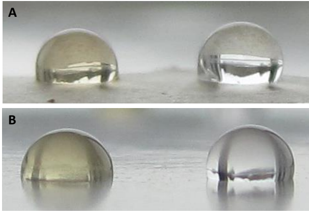
Fig. 28. Liquid droplets collected from P3 (left) and water (right) dropped onto (A) vegetative mycelium and (B) parafilm (each 5 µl volume) indicating different acute angles of attachment to the hydrophobic surfaces. Less acute means more hydrophobic.
