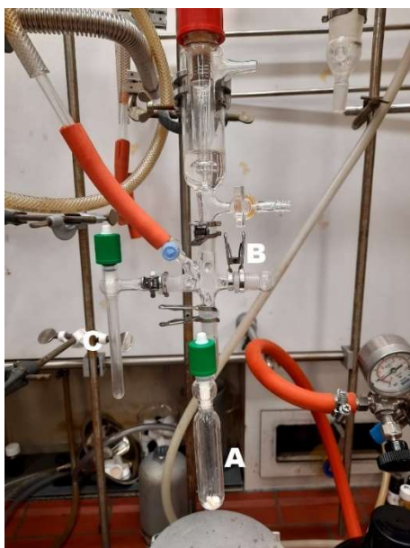
Figure 5.11: Reaction setup for the formation of ^{15}\text{NO} upon reduction of \text{Na}^{15}\text{NO}_2 with \text{FeSO}_4 and \text{H}_2\text{SO}_4 . A: Reaction flask, B: Transfer line, C: Condensation flask.
