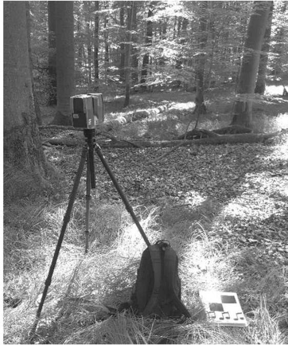
**Figure 1.3:** *Faro Focus 3D terrestrial laser scanner installed on a tripod 1.3 m above ground. An example of the used chessboard targets lies next to the laser scanner. The targets were attached to stems and served as reference points, when multiple scans were merged into one point cloud.*
