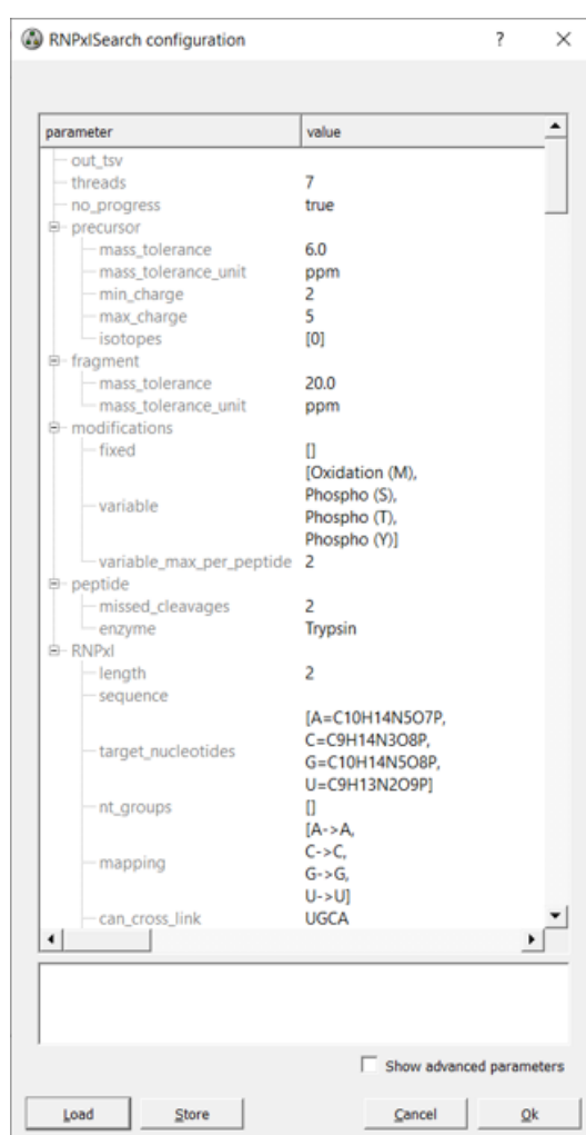
Figure 12: Settings of the RNP xl search node used to identify CSMs. Notice that the MS1 precursor variance was set stringently to 6 ppm to ensure accurate precursor masses. Precursors of charge 2-5 were triggered for an MS2 recording event. MS2 precursor variance was set conservatively to 20 ppm. Additionally, phosphorylation on S, T, and Y, as well as methionine oxidation were allowed as peptide modifications. Lastly, specific adduct masses to peptide fragments corresponding to cross-linked nucleotides were tabulated according to their respective chemical crosslinker in tables found in section 13.1.2.
