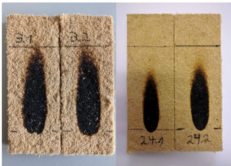
**Figure 7:** Fire performance according to EN ISO 11925-2 (2010) of WFIB made of 100\_birch (left) and of 100\_spruce (right) with 5 wt% pMDI.
