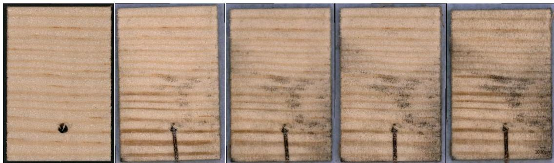
**Figure 5: Mould growth classes from 0 (left) to 4 (right).**
