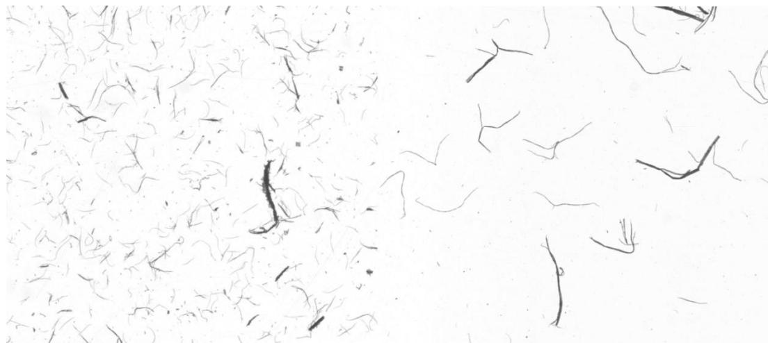
**Figure 1: Scanned particles of single-species ash fibres (“100\_Ash”) on the left side and the industry reference on the right side.**
