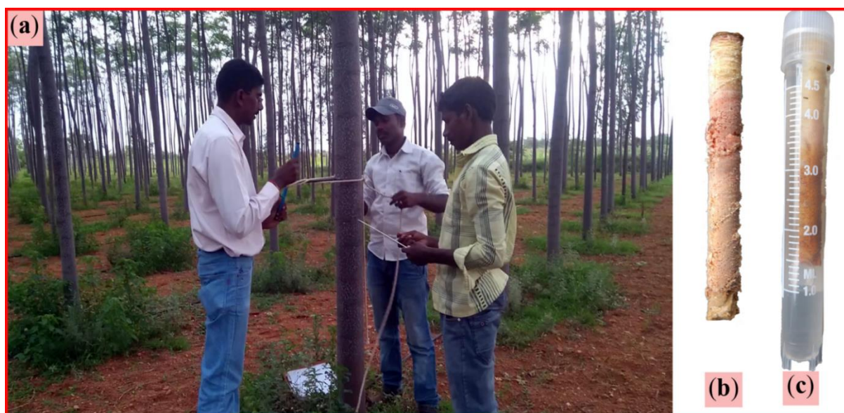
Fig. 3.3. Extraction of stem cores in the field using an increment borer having 5.15 mm inner diameter (Haglöf, Sweden) (a). Extracted wood core(s) (b) were preserved in 50% ethanol for wood anatomical studies (c).
