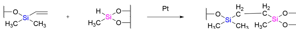
Fig. 3.2: Hydrosilylation reaction scheme. Polydimethylsiloxane is formed through a reaction of a pre-polymer component ( e.g. , dimethylvinyl-terminated dimethylsiloxane) with a component in the curing agent ( e.g. , dimethyl methylhydrosiloxane). This reaction is catalyzed by an active platinum-catalyst. [111,114]
