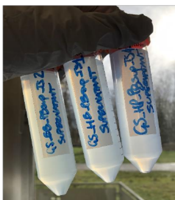
Figure S7. PB milled, tip sonicated and centrifuged EB-NS, HB-NS and HP-NS Self-taken photograph of the fully exfoliated samples, i.e. the final NS batches that underwent complete morphological and photophysical characterization.
