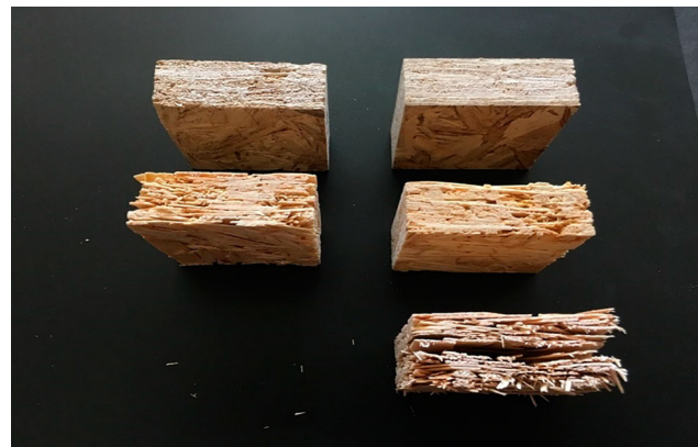
Figure 6. Representative samples of SBs panels from kiri, pine, beech (top to bottom) with a target density of 300 kg m -3 (left side) and 400 kg m -3 (right side).
