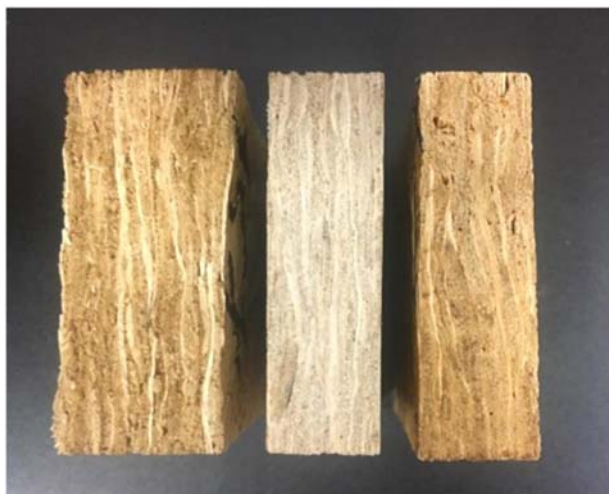
Figure 1. Photo of representative SB test specimens before (untreated control, middle) and after assessing irreversible thickness swelling (ITS) at 1 h vacuum, immersion in water for 96 h and drying; left: panel produced with HMW-PF; right: panel produced with LMW-PF.
