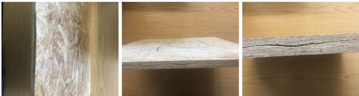
Figure 2 Blisters of kiri strand board after hot pressing and burned board surface
