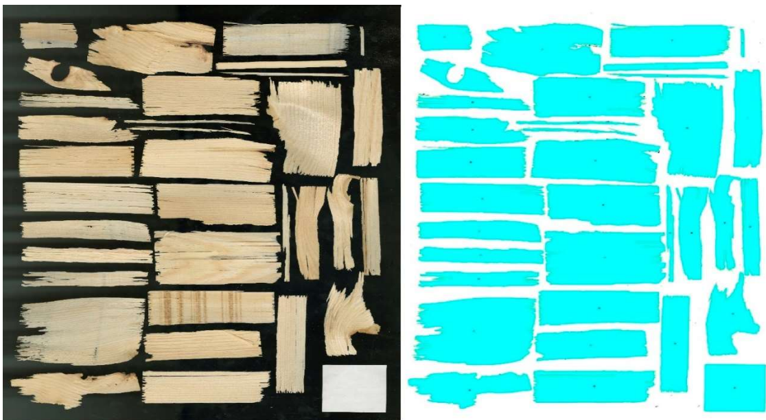
Figure 1 Example for the scanned image before (left) and after (right) segmentation
