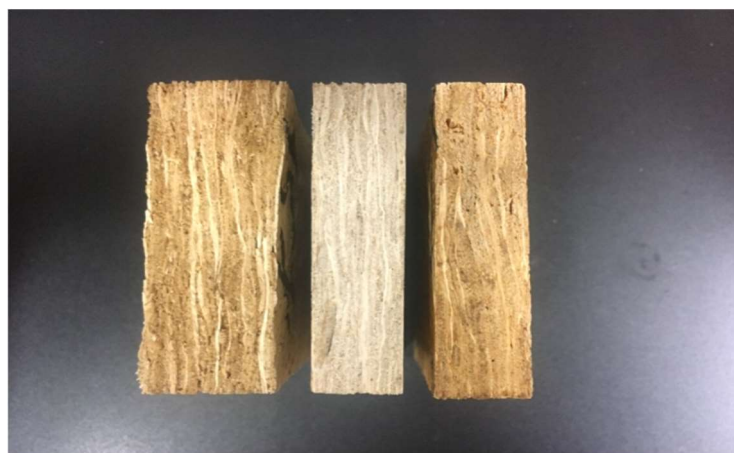
Figure 11 Irreversible thickness swelling SBs samples with high molecular weight PF (left); low molecular weight PF (right) after vacuum at the first hour, then immersion in water for 24, 48, 96h and dried 24h for each temperature 40 0 C, 60 0 C, 80 0 C and at 103 0 C until certain mass; initial thickness (middle).
