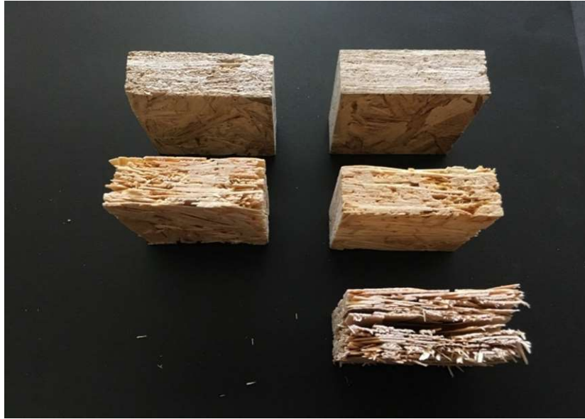
Figure 6 Representatives samples of SBs panels from kiri, pine, beech (top to bottom) with a target density of 300 \text{ kg m}^{-3} (left side) and 400 \text{ kg m}^{-3} (right side)
