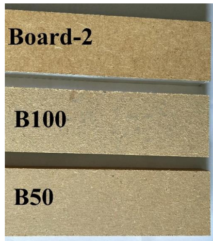
Figure 5.3: Uncoated industrial Board-2 fibreboard and recycled MDF panels (B100 and B50) produced using recovered fibres obtained by the disintegration of Board-2 (RF2).
