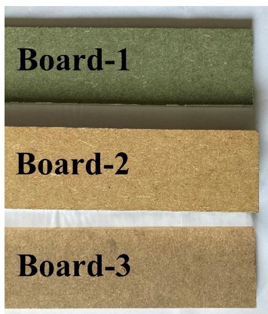
Figure 5.1: Uncoated industrial fibreboards used for the thermo-hydrolytic disintegration process.
