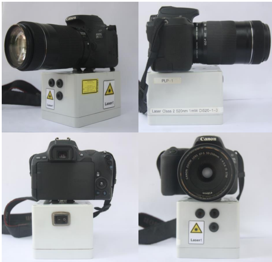
Figure A2.1. Apparatus for Parallel Laser Photogrammetry (PLP) used in the study, seen from different angles. The apparatus, also referred as PLP system, consisted of a camera and a laser box with three lasers and a switch. Batteries were allocated inside the laser box. Horizontal and vertical lasers were separated by 20 millimetres.
