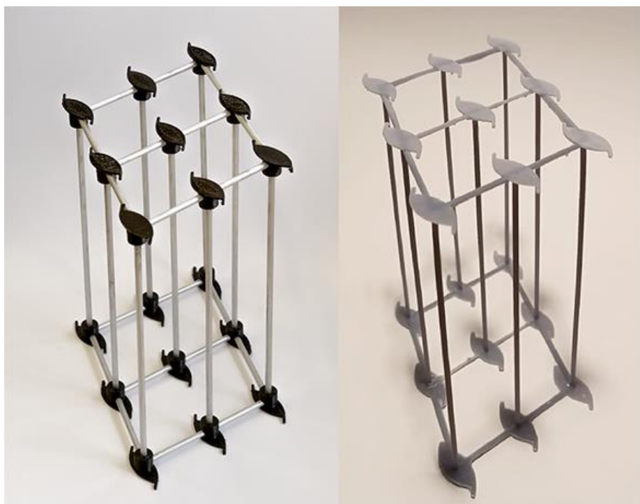
Figure 2-23: Small-scale prototypes of space group models. Left: Model assembled from aluminium rods and custom parts made with a filament 3D printer. Right: Whole model printed with a resin 3D printer.
