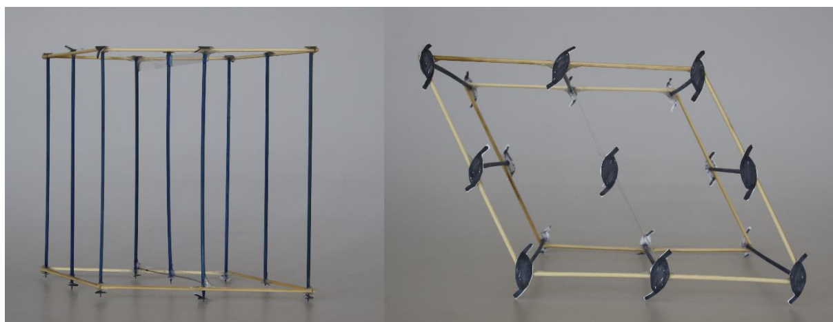
Figure 5-24: Prototype model of space group P2_1 . Left: Arbitrary direction. Right: View along crystallographic b axis.
