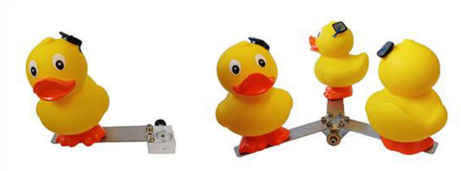
Figure 2-18: Left: Object mount designed for the screw axis models holding a rubber duck. Right: Special mount for the model of a 6_3 screw axis holding three rubber ducks at equal height and in 120^\circ angles.
