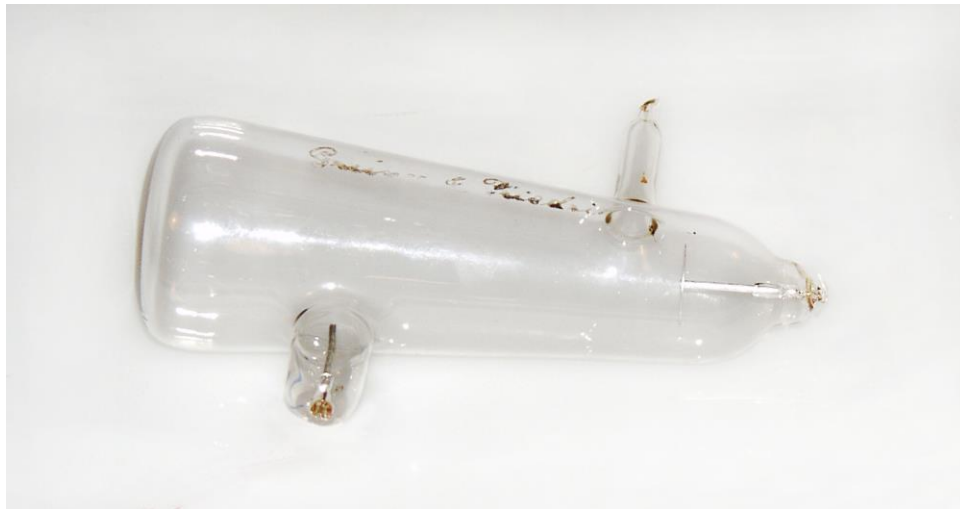
Figure 1-1: Cathode ray tube produced by Greiner & Friedrichs around 1896, similar to the ones W. C. Röntgen had at his hands. On the right side of the tube a disc cathode is embedded, on the bottom left the anode is connected. Photograph kindly provided by the Deutsche Röntgen-Museum Remscheid, Photographer: Christina Falkenberg.
