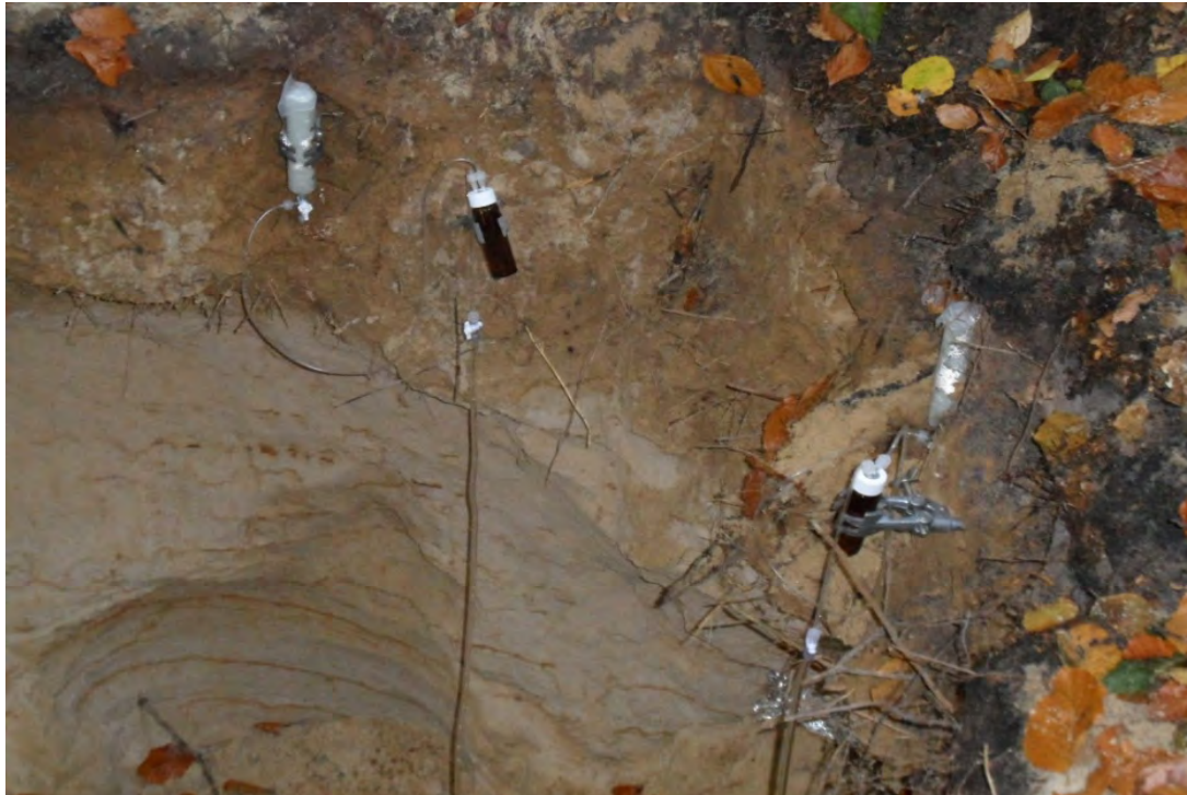
Figure 1 Exemplified collection of root exudates the layer of 20-50 cm depth. Sampling cutvettes (briefly uncovered) with embedded roots and associated sterile collection vessels attached to terminal zones of root strands.
