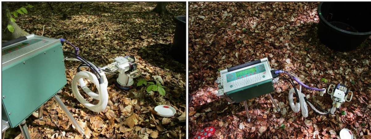
Figure 2.1 Soil respiration measurements with a LI-6400 and a soil CO 2 flux chamber (LI-6400-09). Chamber was stabilized by PVC soil collars and placed 1 cm above soil surface. A (blue) fine foam gasket ring was placed between soil collar and chamber to avoid disturbance and air leakage. Simultaneous measurement of soil temperature was performed via temperature probe (violet cable).
