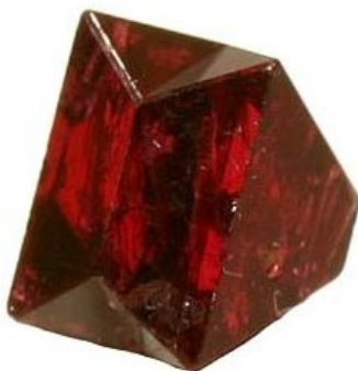
Figure 2.10.: Image of twinning in a \text{MgAl}_2\text{O}_4 spinel gem (see text for reference). Indications for twinning, i.e. similar shapes of well-faceted particles, were also observed for \text{LiMn}_2\text{O}_4 in this work.
