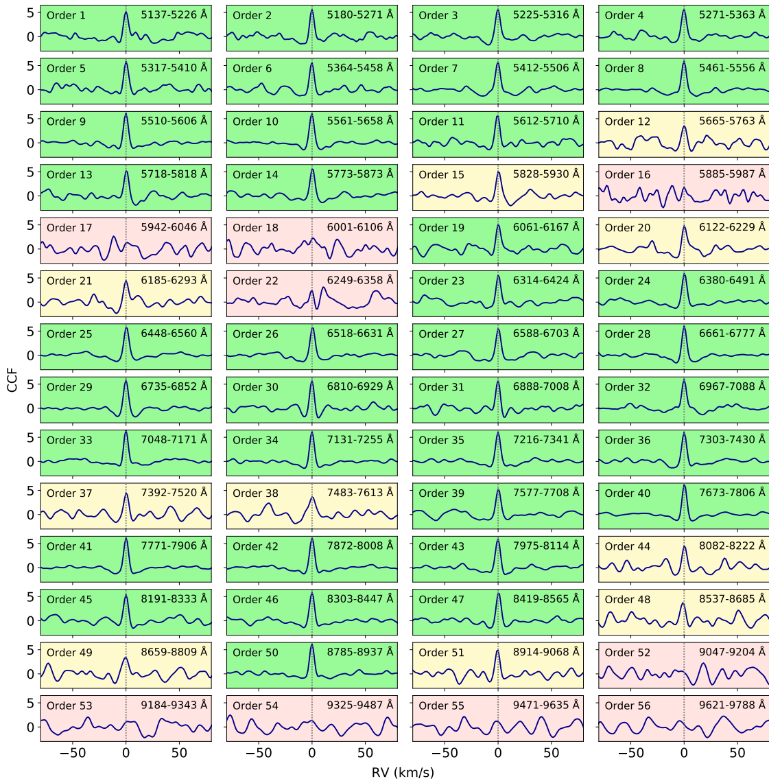
Figure 2.11.: CCFs between the TiO transmission model and the high-resolution spectrum of Barnard's star for CARMENES. The x -axis represents the radial velocity offset from the stellar rest frame; the y -axis measures the CCF in units of standard deviation. The yellow and green shaded panels indicate the spectral orders with a CCF peak greater than three and five standard deviations, respectively. Red shaded panels represent spectral orders not showing any correlation.
