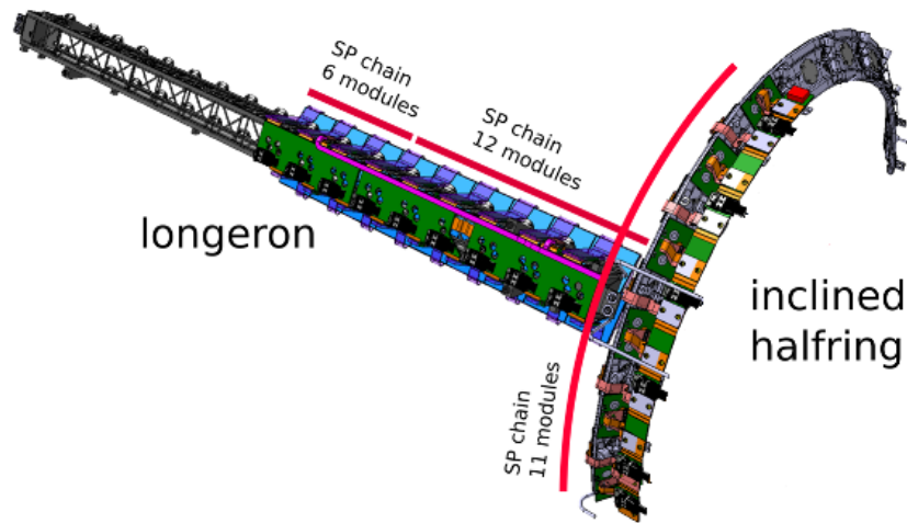
Figure 8.20: Sketch of the RD53A demonstrator setup.
