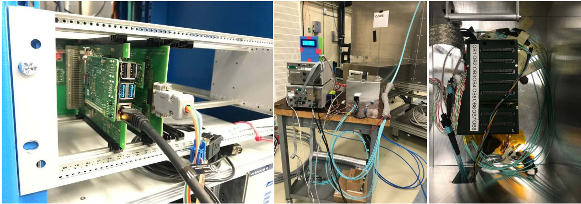
Figure 8.21: Left: The MoPSHUB 4beginners, housing the RaspberryPi and a CIC card. Middle and right: Optobox with seven optobards, including power board, connector board, housing and cooling plate.
