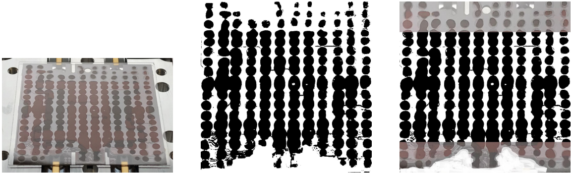
Figure 7.14: Analysis of the adhesive pattern after a curing time of 15 min without releasing vacuum on the flex jig. Left: Gluing pattern as seen from the side for contrast between adhesive covered area and free space. Middle: Transformation of the full image with the python script and a picture editing programme. Right: Definition of an analysis area.
