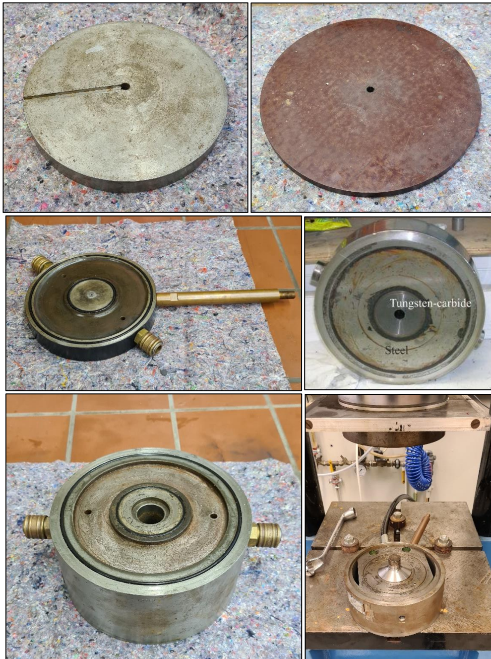
Figure 16: Components of a piston cylinder press. spacer (top left), insulation plate (top right), top plate (middle left), bomb (middle right), bridge (bottom left) and master ram (bottom right).
