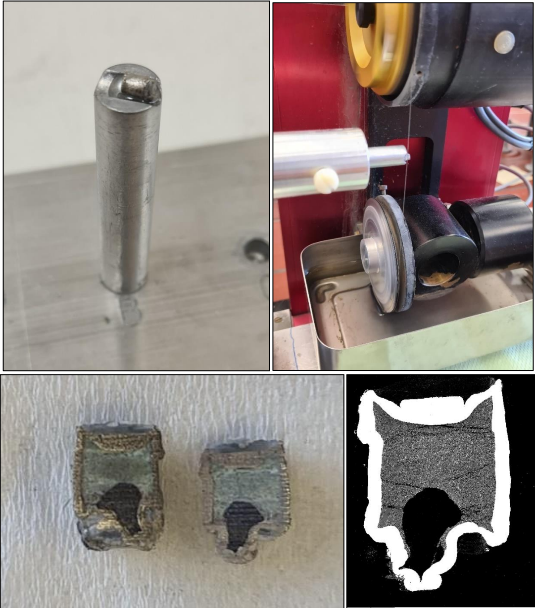
Figure 54: Specimen capsule attached to specimen holder with Crystal Bond (top left), sawing process with diamond-coated wire (top right) and split specimen capsules before polishing (bottom left) and in the SEM (bottom right).
