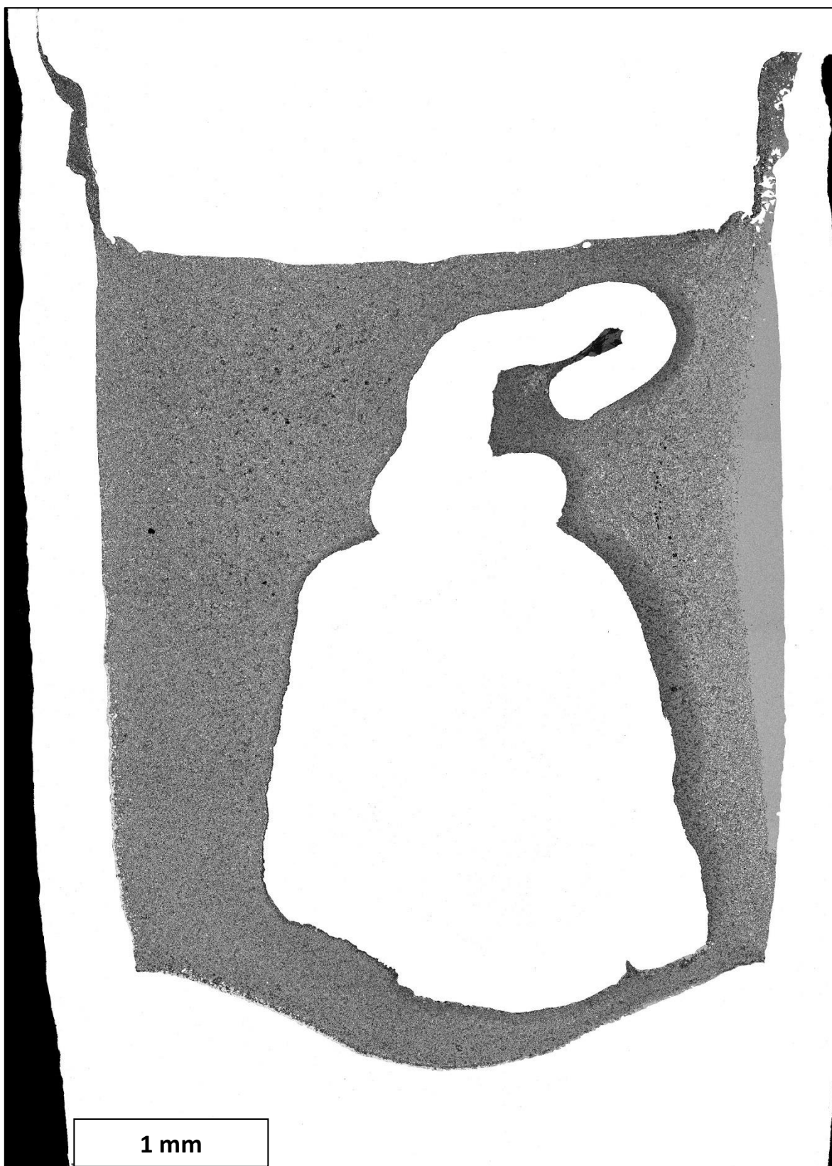
Figure 112: General view of sample LPUM 050-1 with outer iron capsule (white) and inner platinum capsule with buffer material (white).
