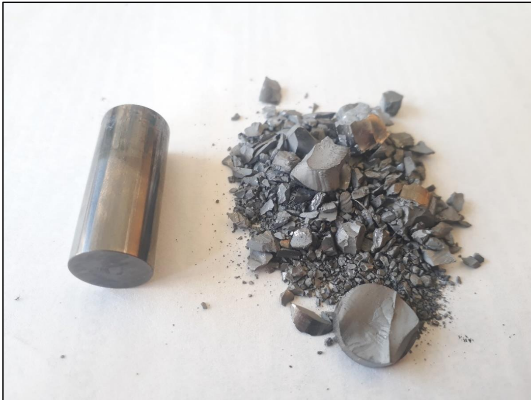
Figure 24: Material failure of the piston due to the high loads during the experiments. Left: intact piston. Right: condition after blow-out
