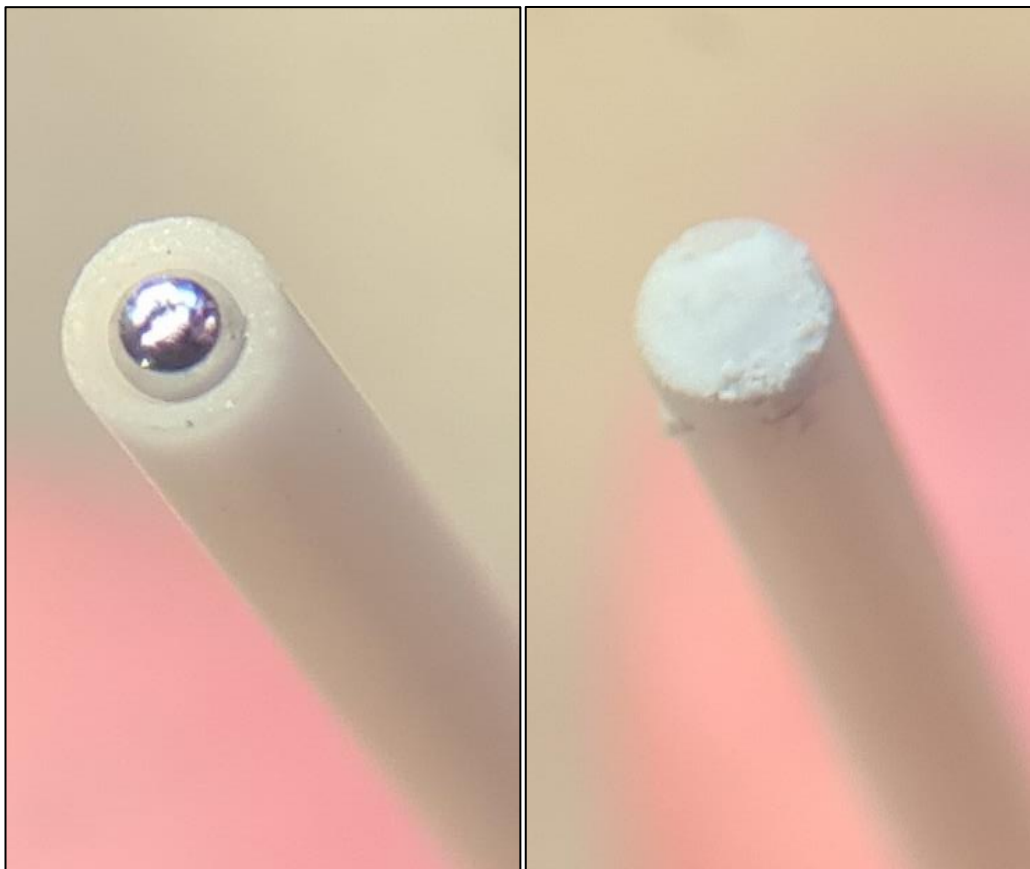
Figure 39: Thermocouple with recessed weld bead (left) and after cementing (right).
