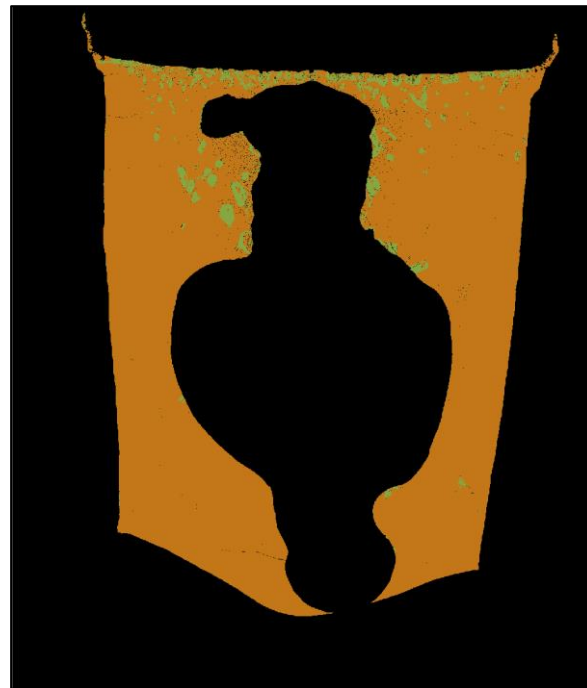
Figure 104: Separation by grey values of sample 100-1 using MATLAB. Original image (top) and constructed image from the separation (bottom).
