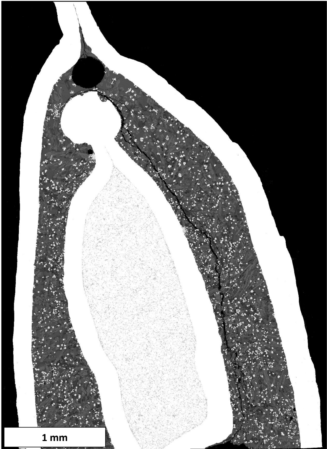
Figure 120: General view of sample LPUM 030-1 with outer and inner platinum capsule (white). The buffer material can be seen as a shadow in the inner platinum capsule.
