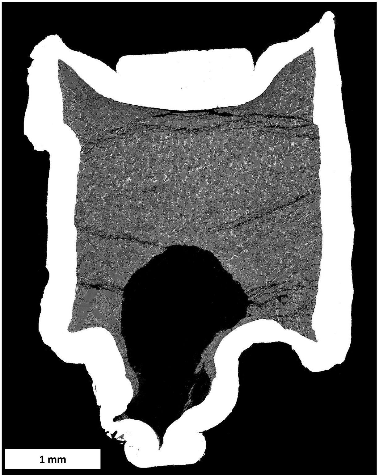
Figure 69: Overview image of sample LPUM 300-1 with outer platinum capsule (white) and carbon as buffer material (black in contact with the sample).
