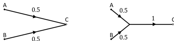
Figure 4.1: Sketch of Wasserstein-1 transport (left) and branched transport (right) from \frac{1}{2}(\delta_A + \delta_B) to \delta_C .
