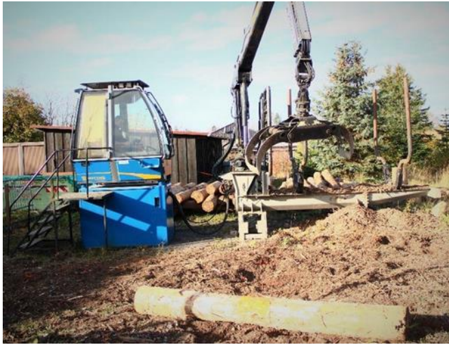
Figure 3: Rottne-F10-based forwarder simulator used in the study (Image: Hartsch).
