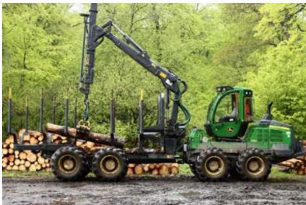
Figure 8: John Deere Forwarder 1210 G used in the study (Image: Hartsch).
