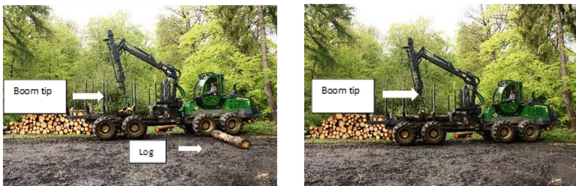
Figure 10: Forwarder at start (left) and end (right) of loading cycle.
