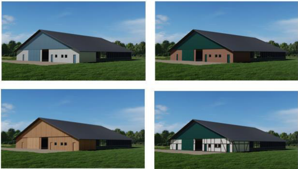
Figure 1. Various materials and different colored façades used for the exterior of the barns (gray-blue trapezoidal sheet metal façade, wooden façade, red clinker brick façade, white half-timbered façade)
