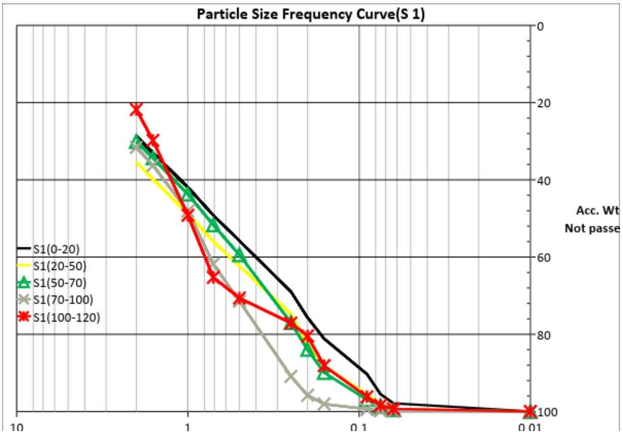
Figure 10.1: Particle size Frequency cure of Sample no.1, ( S1 )
