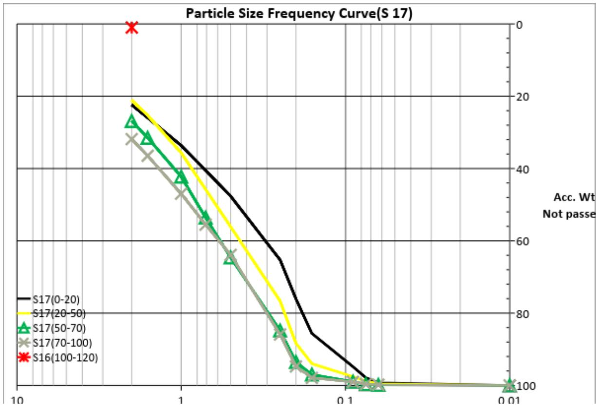
Figure 10.17: Particle size Frequency cure of Sample no.17, ( S17 )
