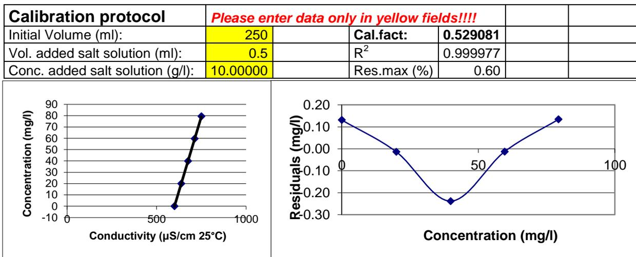
Figure 4.4: Calibration Curve of Auja Spring, Experimental Measurement of Spring discharge, June, (2013)
