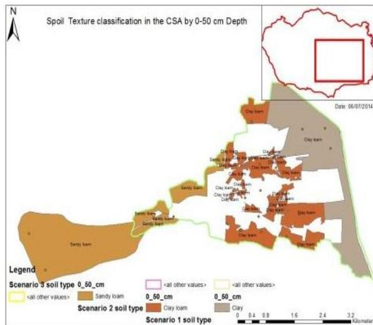
Figure 3.15a: Soil classification based on Soil Texture analysis in the CSA
