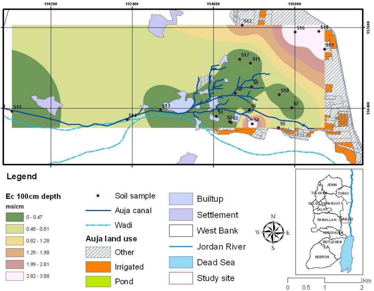
Figure10.28: Electrical conductivity Value of (70-100 cm) depth at the CSA.
