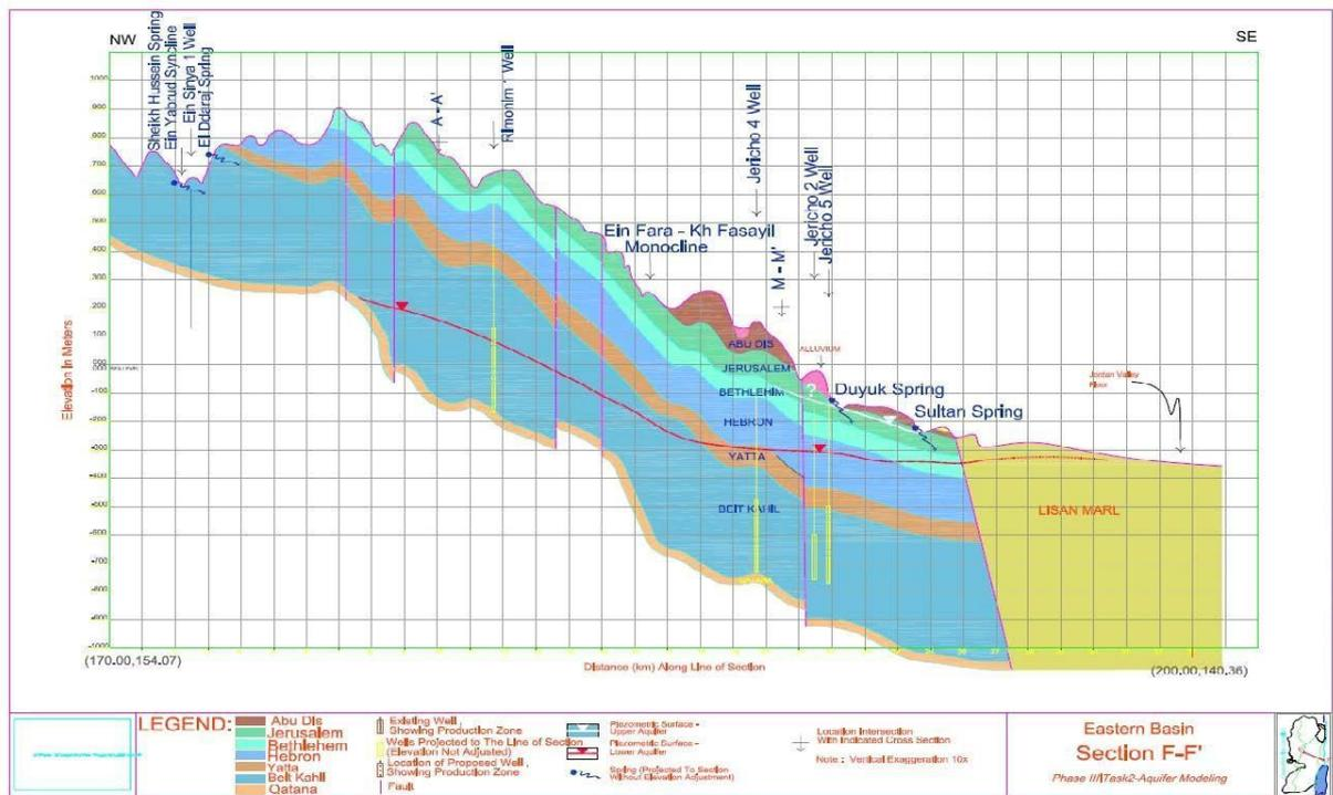
Figure 2.18: Hydrogeological cross section in Jericho area (Ground water Management Model, Task 7, The Jericho Model, CH2MHILL, 2001).
