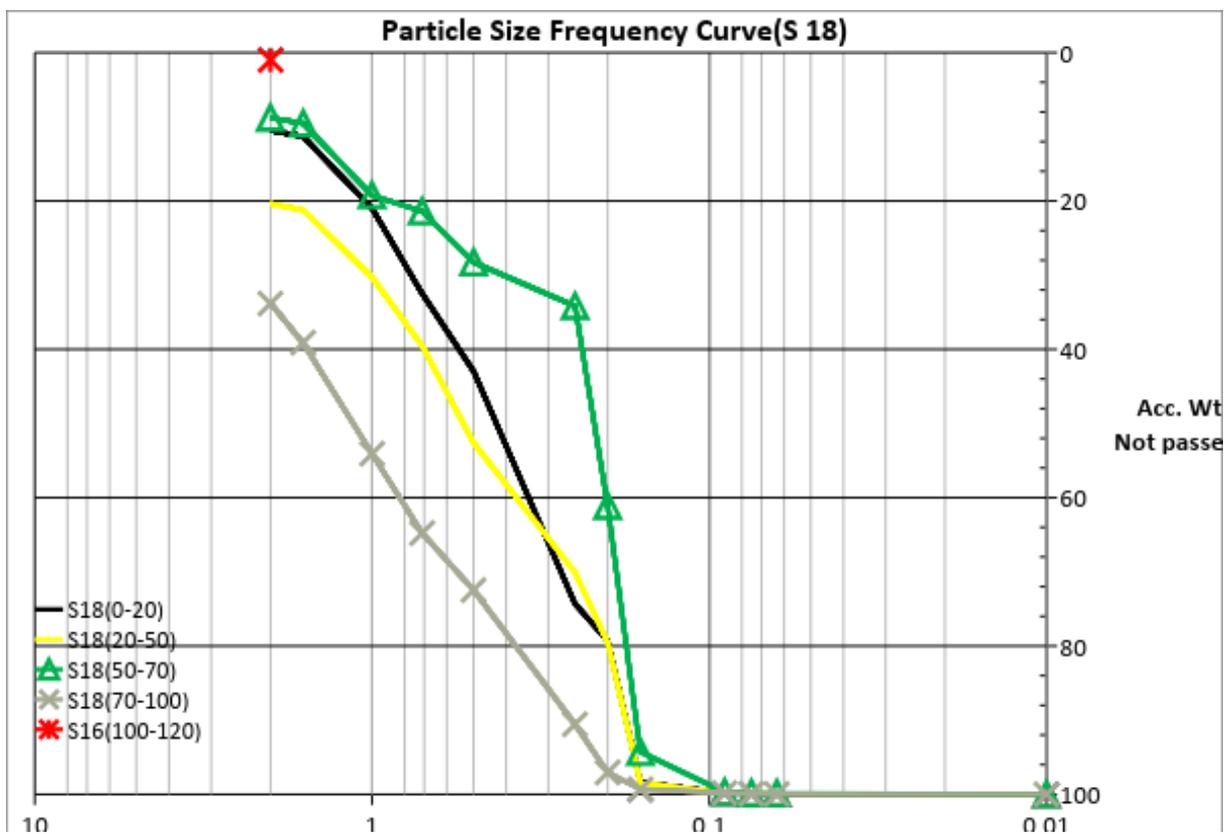
Figure 10.18: Particle size Frequency cure of Sample no.18, ( S18 )
