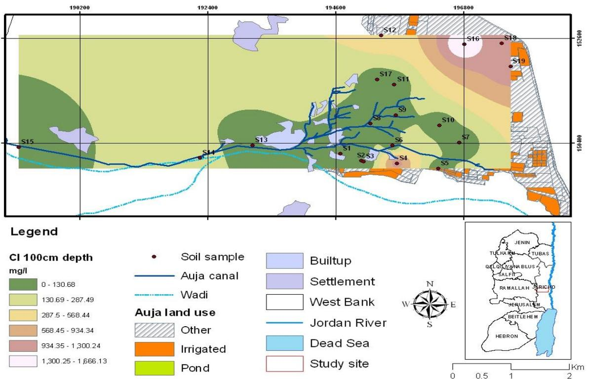
Figure10.23: Chloride concentration of (70-100 cm) depth at the CSA.
