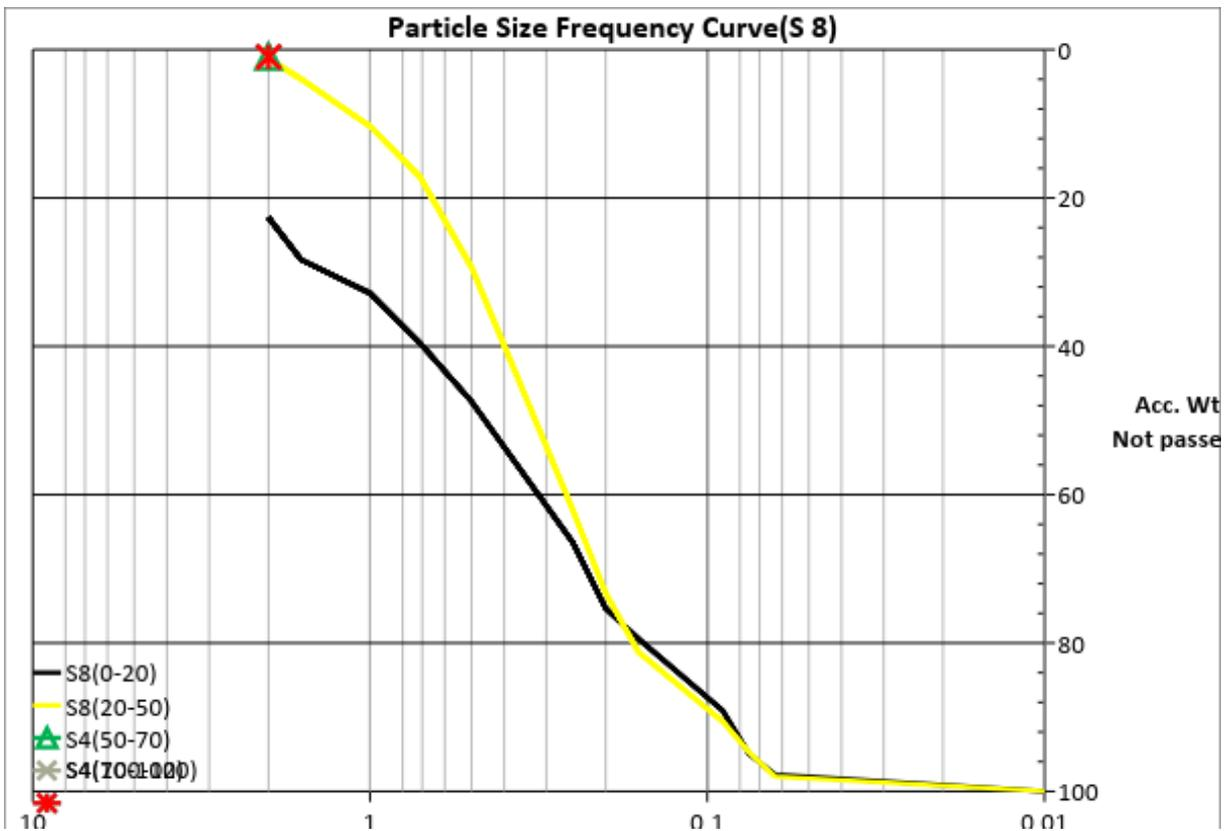
Figure 10.8: Particle size Frequency cure of Sample no.8, ( S8 )
