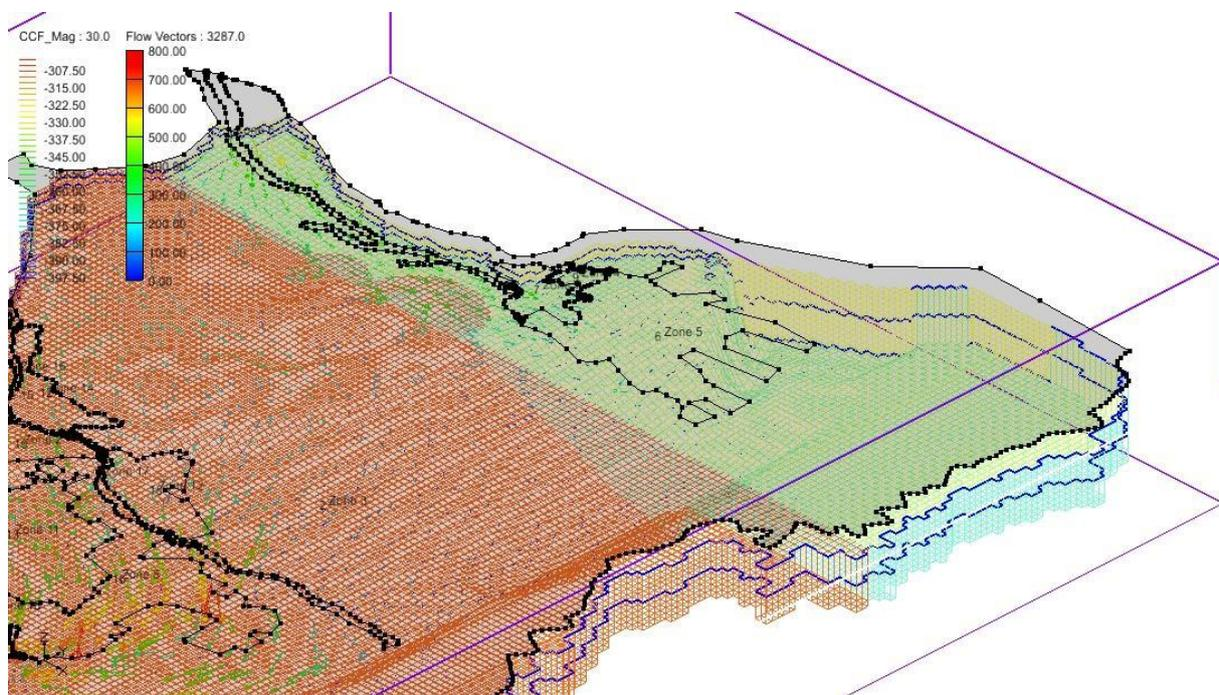
Figure 5.16: Recharge zones in the CSA including the main recharge source.
