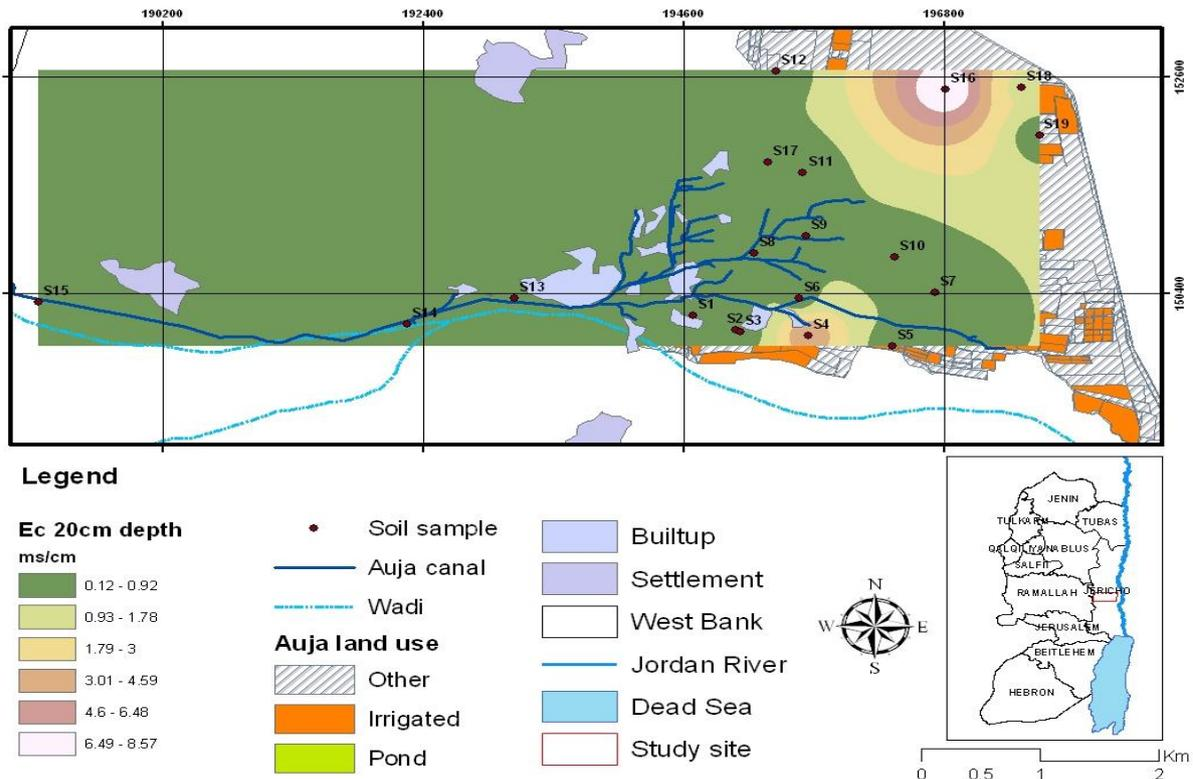
Figure10.25: Electrical conductivity Value of (0-20 cm) depth at the CSA.
