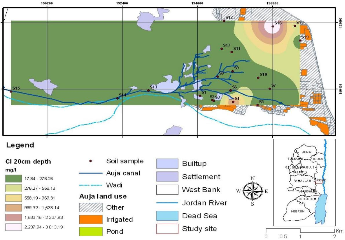
Figure10.20: Chloride concentration of (0-20 cm) depth at the CSA.
