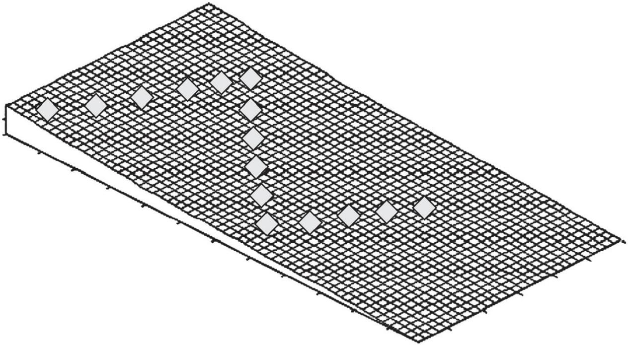
Figure 3.3: Zig-Zag method for selecting soil samples in arid zones.
