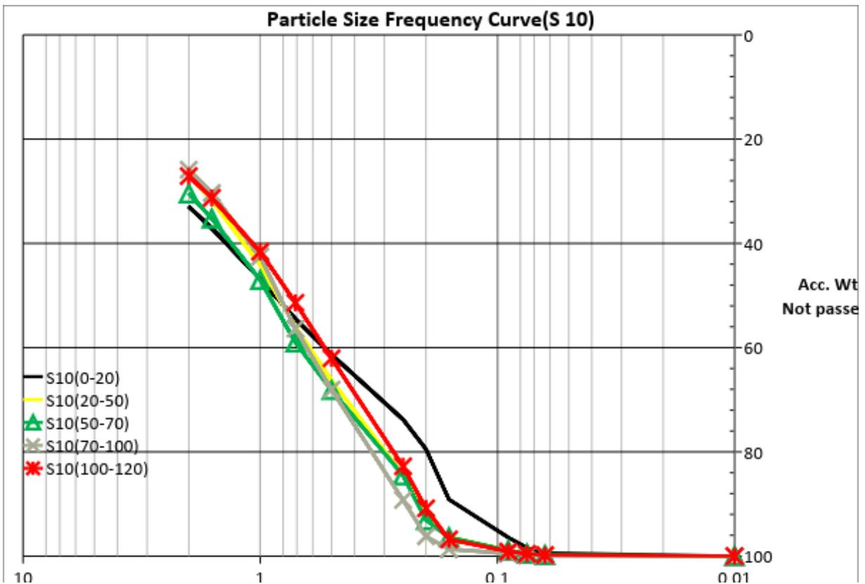
Figure 10.10: Particle size Frequency cure of Sample no.10, ( S10 )
