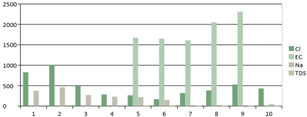
Figure 2.23: Chloride concentration and EC during years 2000-2009 ,well no. 19-15/023.
