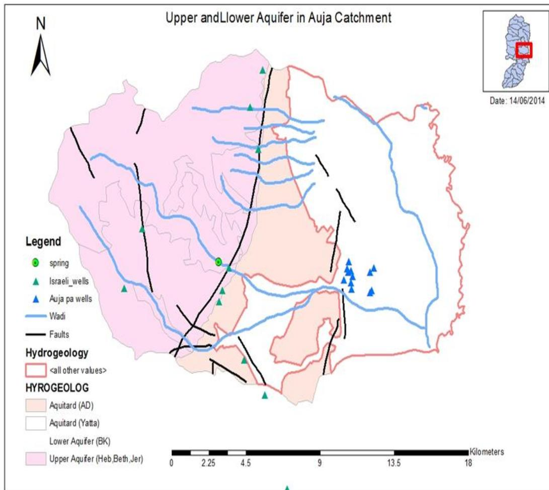
Figure 2.21: Upper and Lower Aquifer in the CSA catchment: the hydrological system.
