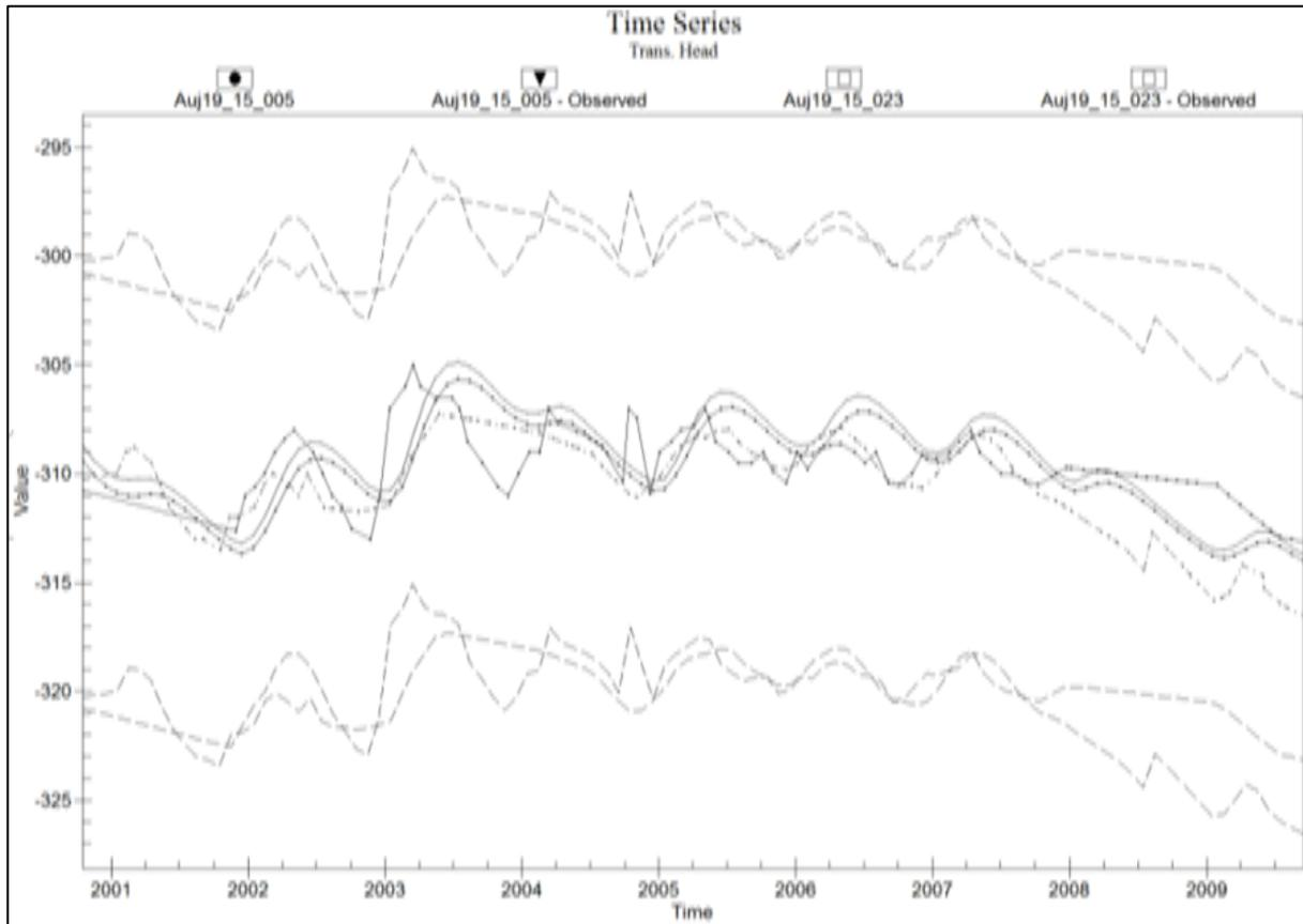
Figure 5.34: Calibration curves with calibration target of wells No. 19-15/005 and Well No.19-15/023 in the CSA.
