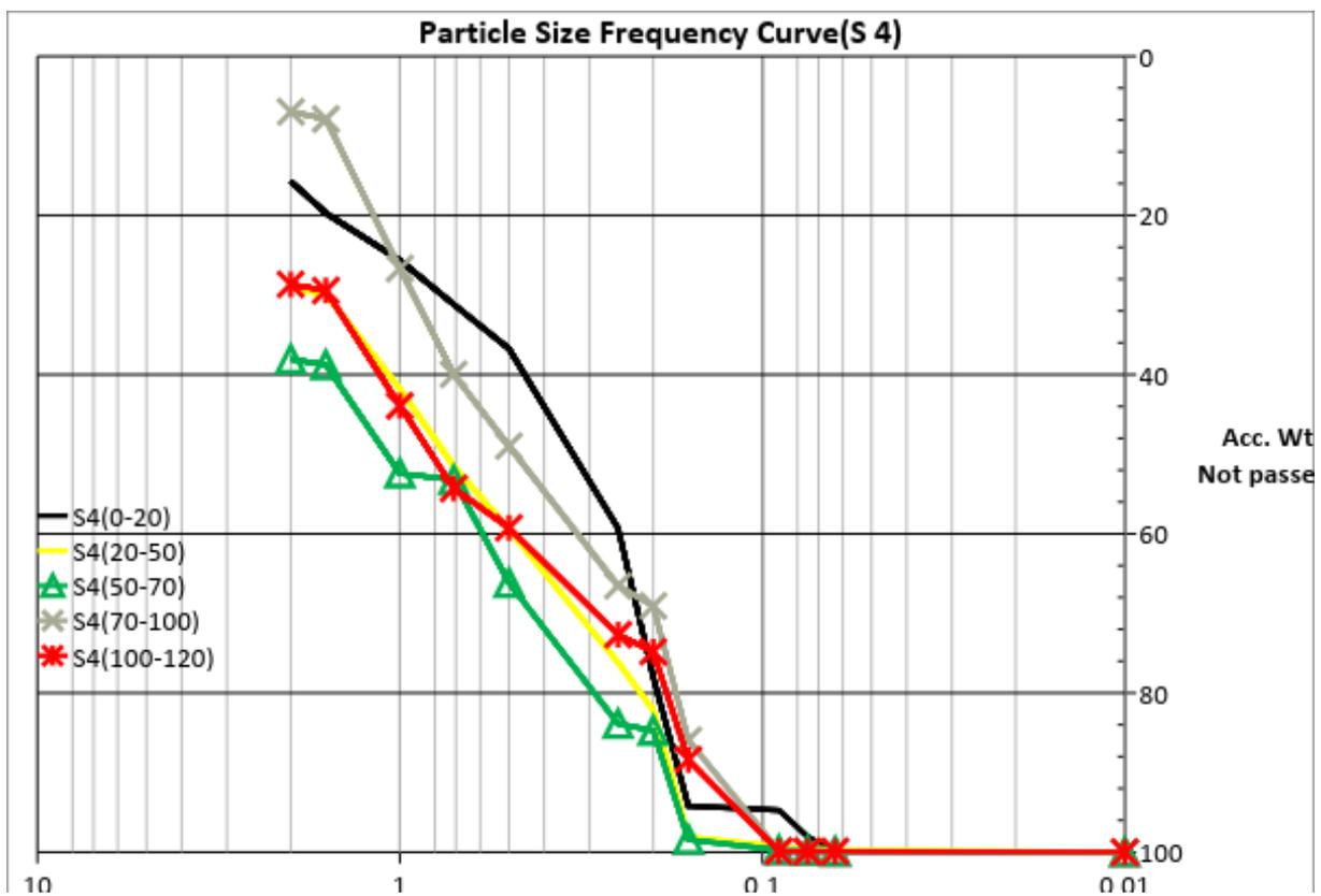
Figure 10.4: Particle size Frequency cure of Sample no.4, ( S4 )
