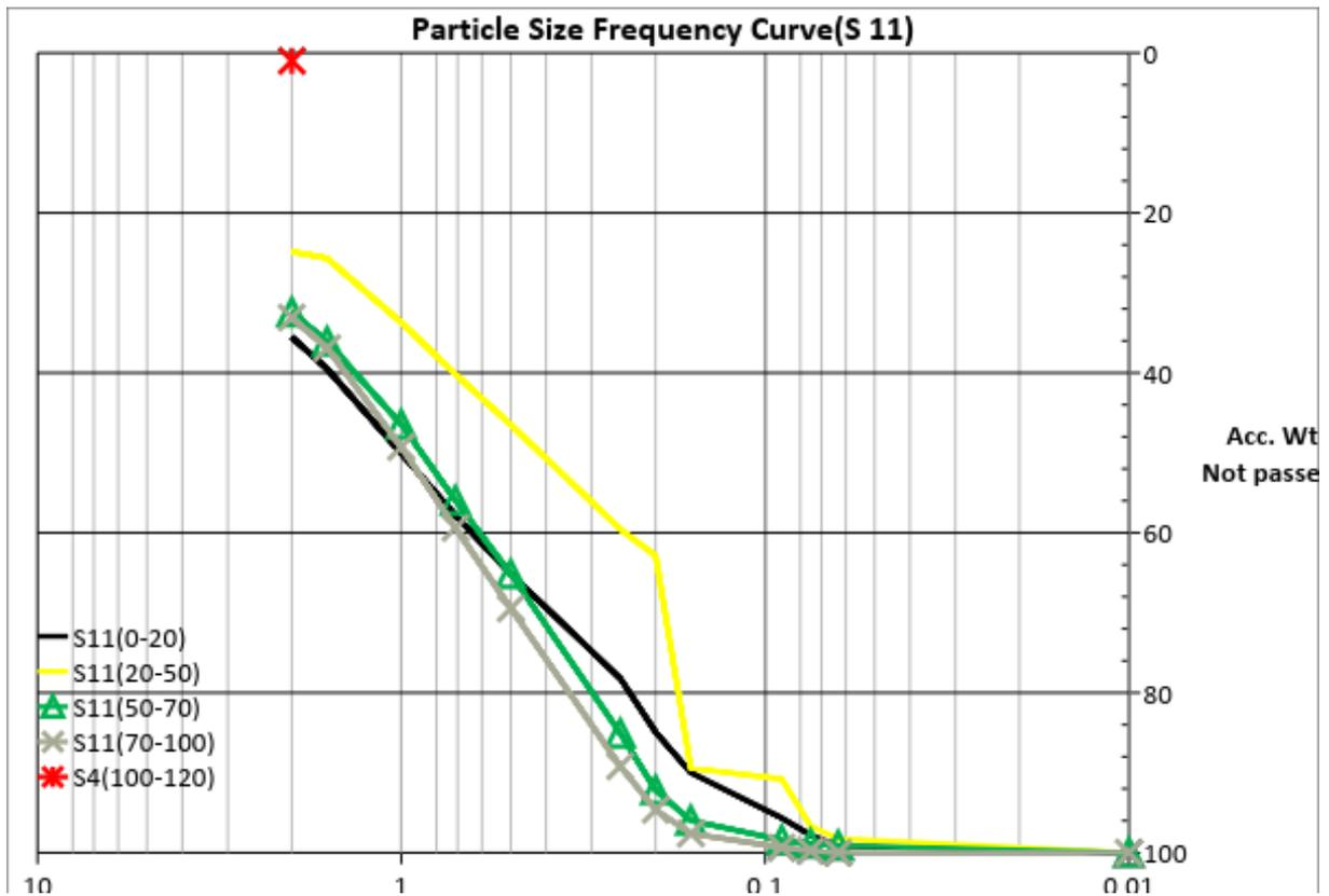
Figure 10.11: Particle size Frequency cure of Sample no.11, ( S11 )
