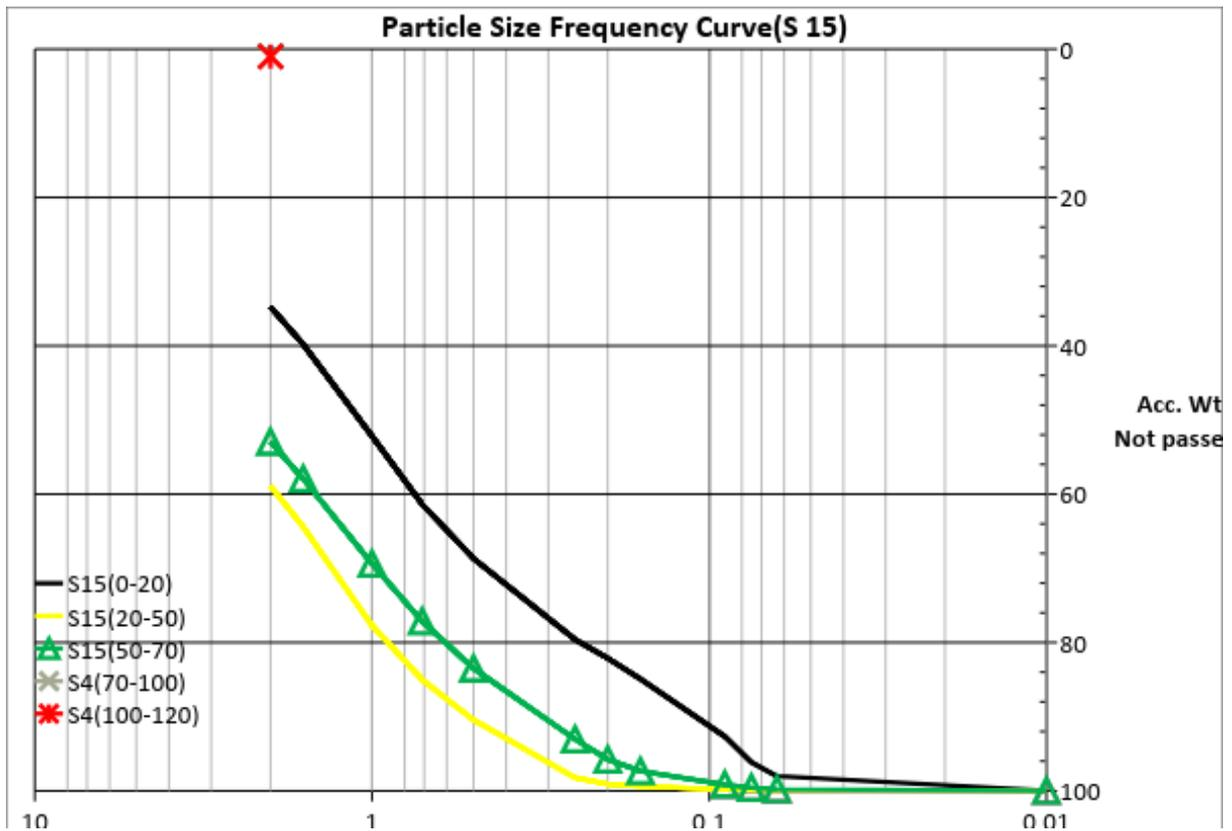
Figure 10.15: Particle size Frequency cure of Sample no.15, ( S15 )
