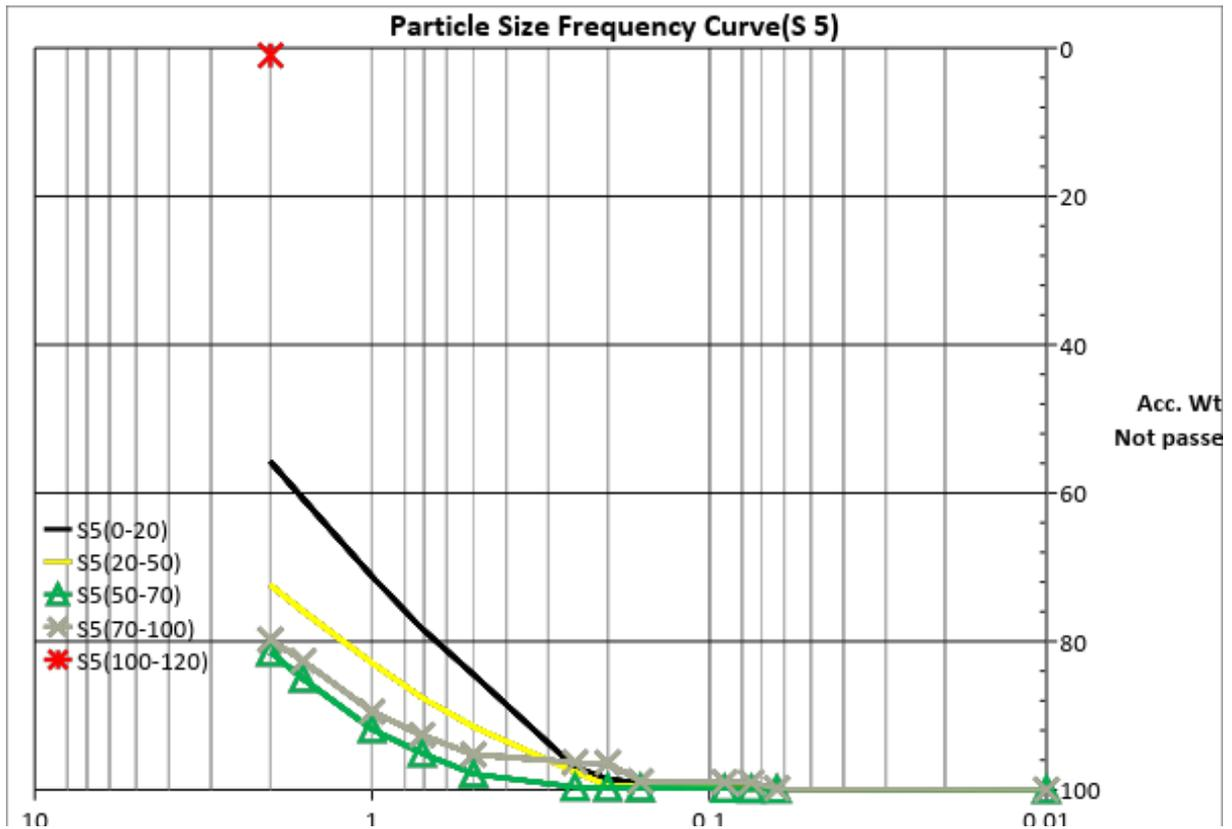
Figure 10.5: Particle size Frequency cure of Sample no.5, ( S5 )
