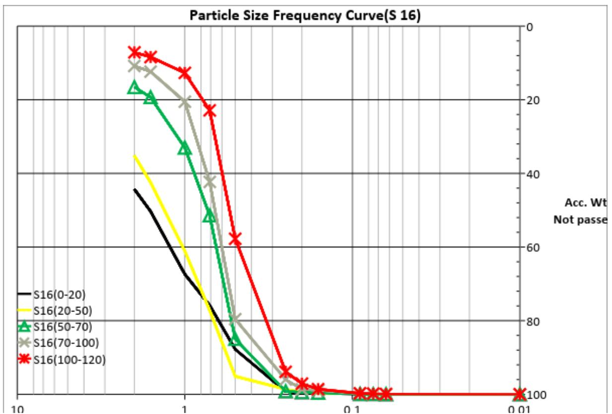
Figure 10.16: Particle size Frequency cure of Sample no.16, ( S16 )
