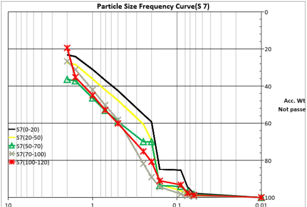
Figure 10.7: Particle size Frequency cure of Sample no.7, ( S7 )
