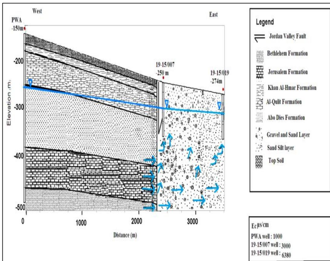
Figure 2.19: Cross section of PWA well to the well no.19-15/019, PWA, Amer Marei, 2013
