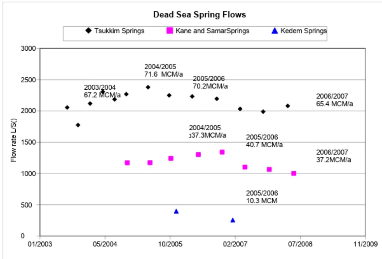
Figure 4.9: Flow rate and spring discharge of Dead sea spring groups during (2003-2009), PWA Data Base, (2011).
