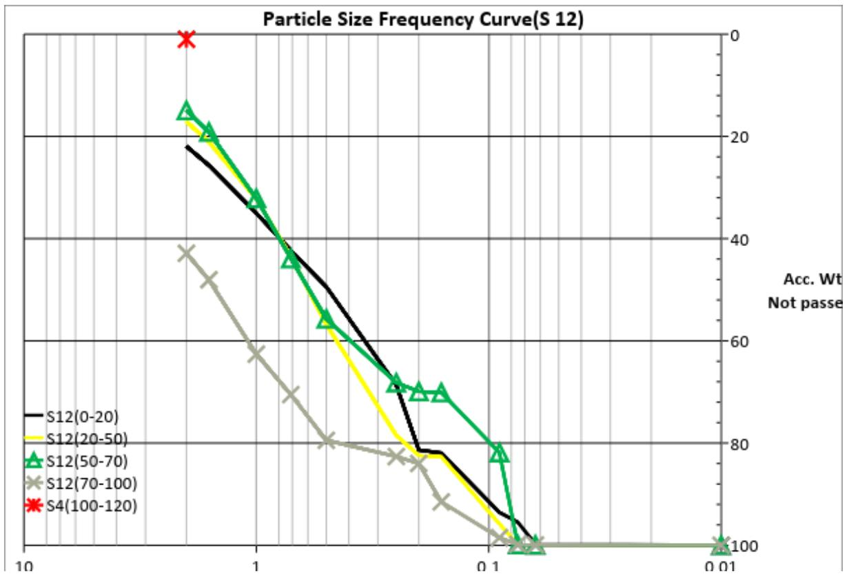
Figure 10.12: Particle size Frequency cure of Sample no.12, ( S12 )
