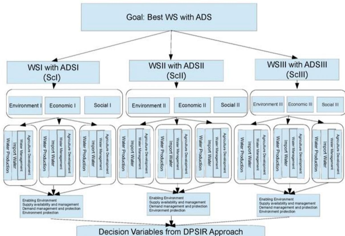
Figure 6.4: Decision Criteria structure which has three sub-criteria levels ,ranking DVs.
