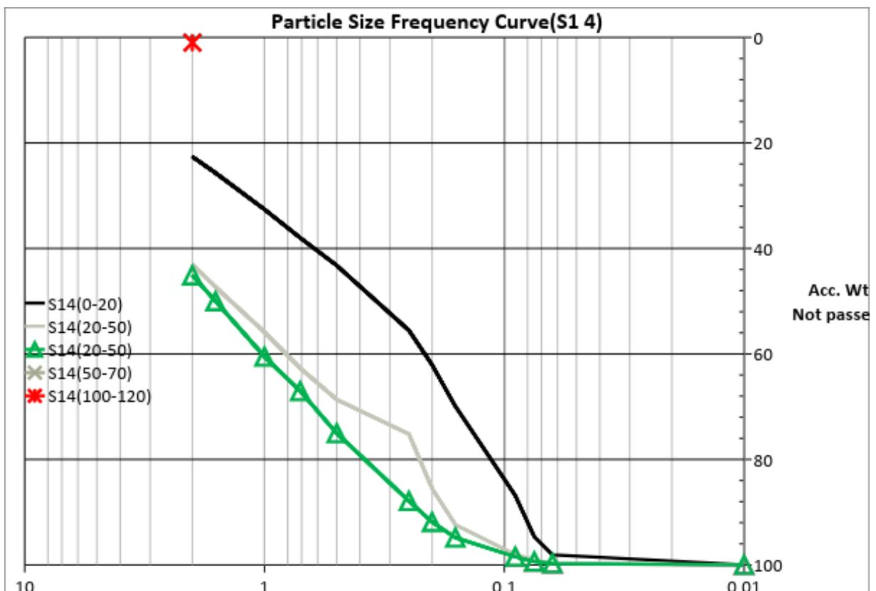
Figure 10.14: Particle size Frequency cure of Sample no.14, ( S14 )
