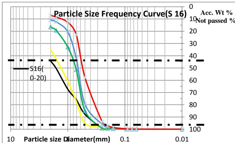
Figure 3.10: PSF-Curve of Site 16 samples with all soil depth profile
