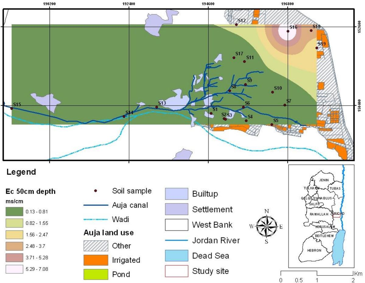
Figure 10.26: Electrical conductivity Value of (20-50 cm) depth at the CSA.
