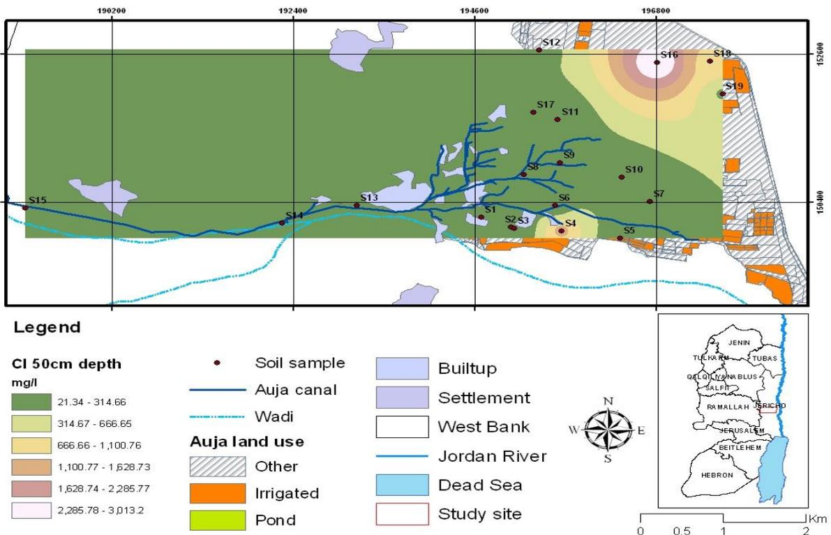
Figure10.21: Chloride concentration of (20-50 cm) depth at the CSA.
