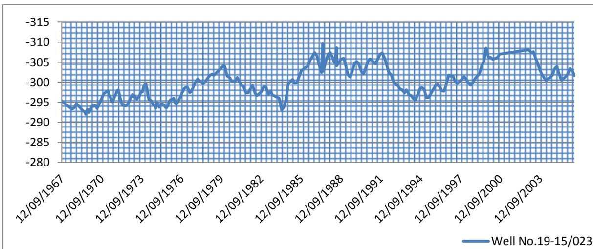
Figure 5.18: Historical data example of well No. 19-15/23, fluctuation from 1967 to 2003.
