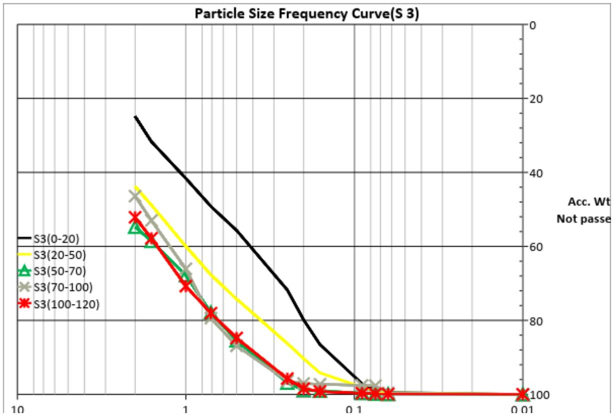
Figure 10.3: Particle size Frequency cure of Sample no.3, ( S3 )
