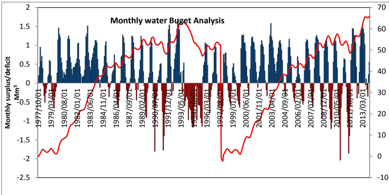
Figure 5.38: Water budget analysis applying MAR and ASR using direct injection and agricultural ponds infiltration in the CSA
