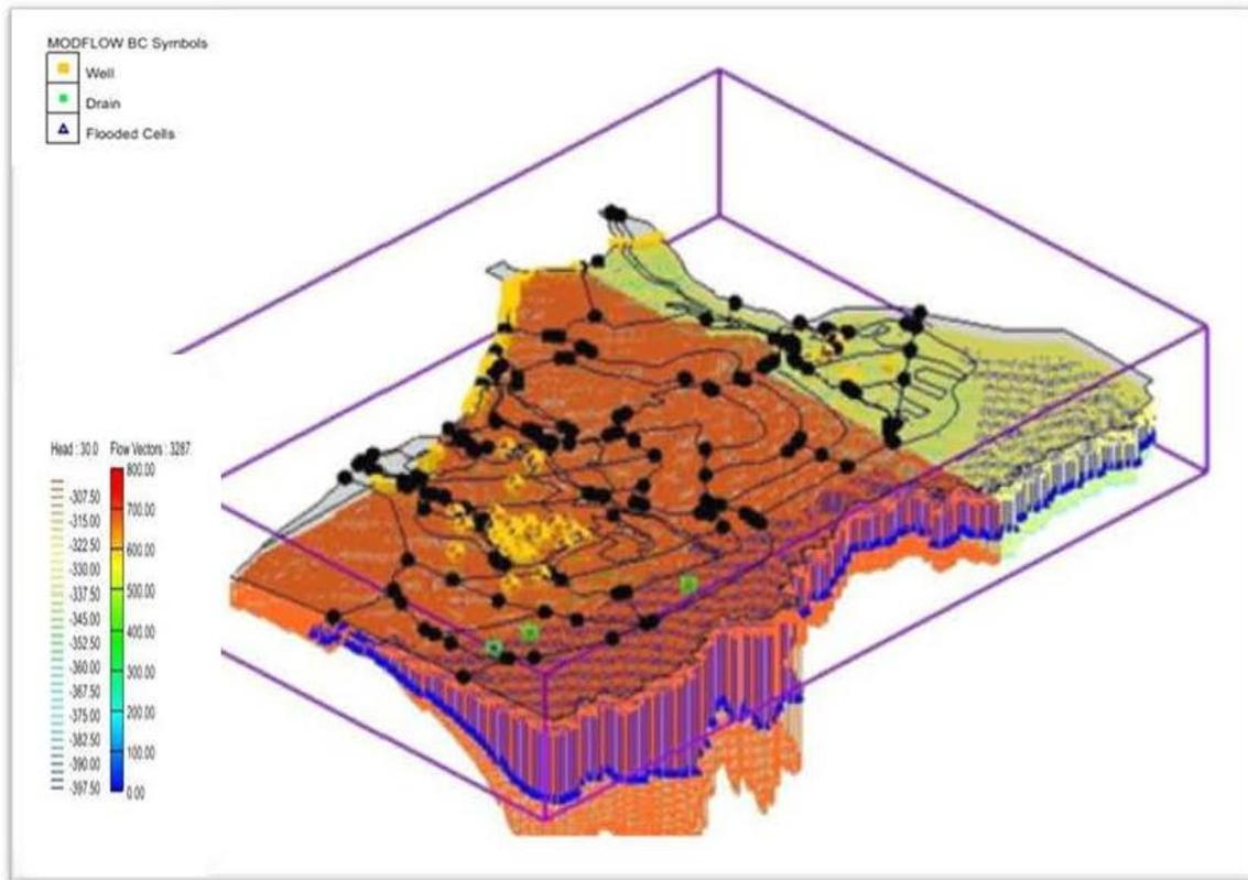
Figure 5.11: Flooded Cells of 2-layer GMS-Modflow Model of the CSA and Jericho Zone
