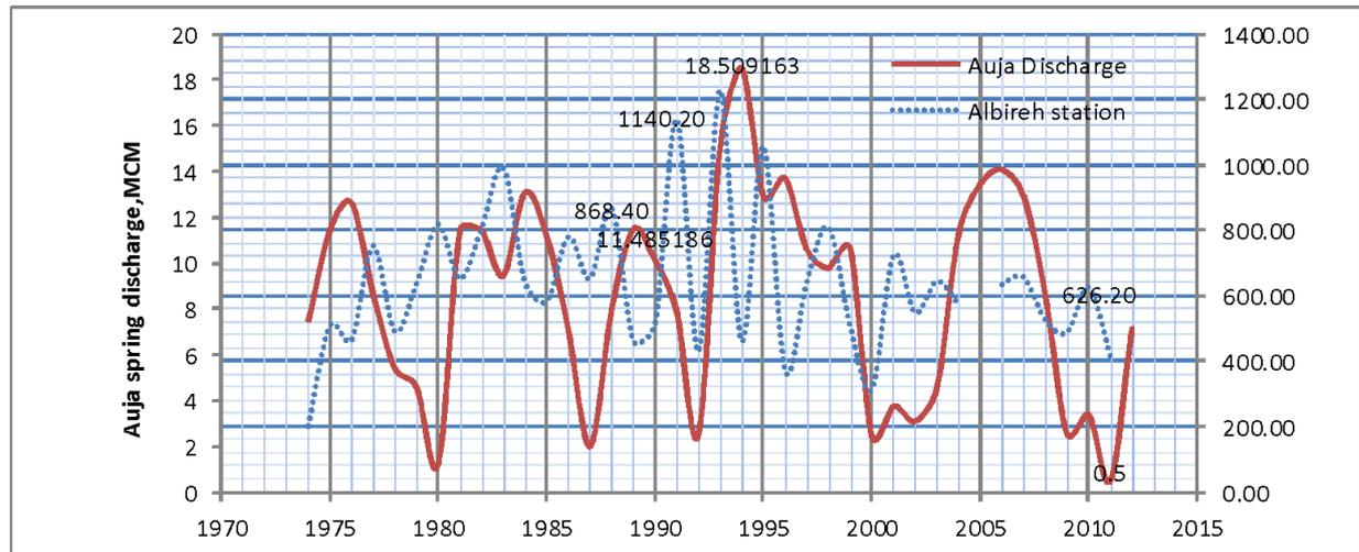
Figure 2.16: Auja Spring fluctuation and precipitation time series (PWA Data base, 2012)
