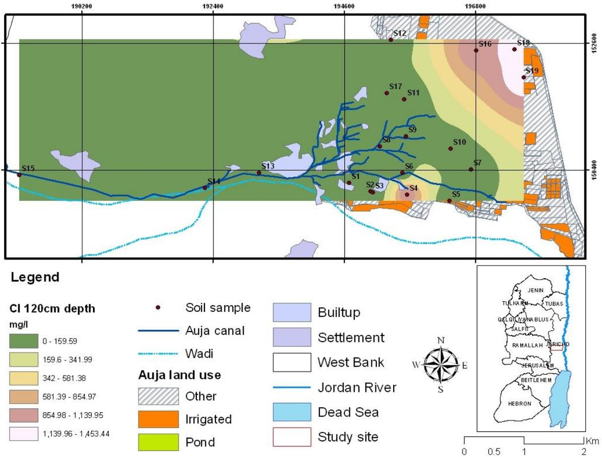
Figure10.24: Chloride concentration of (100-120 cm) depth at the CSA.
