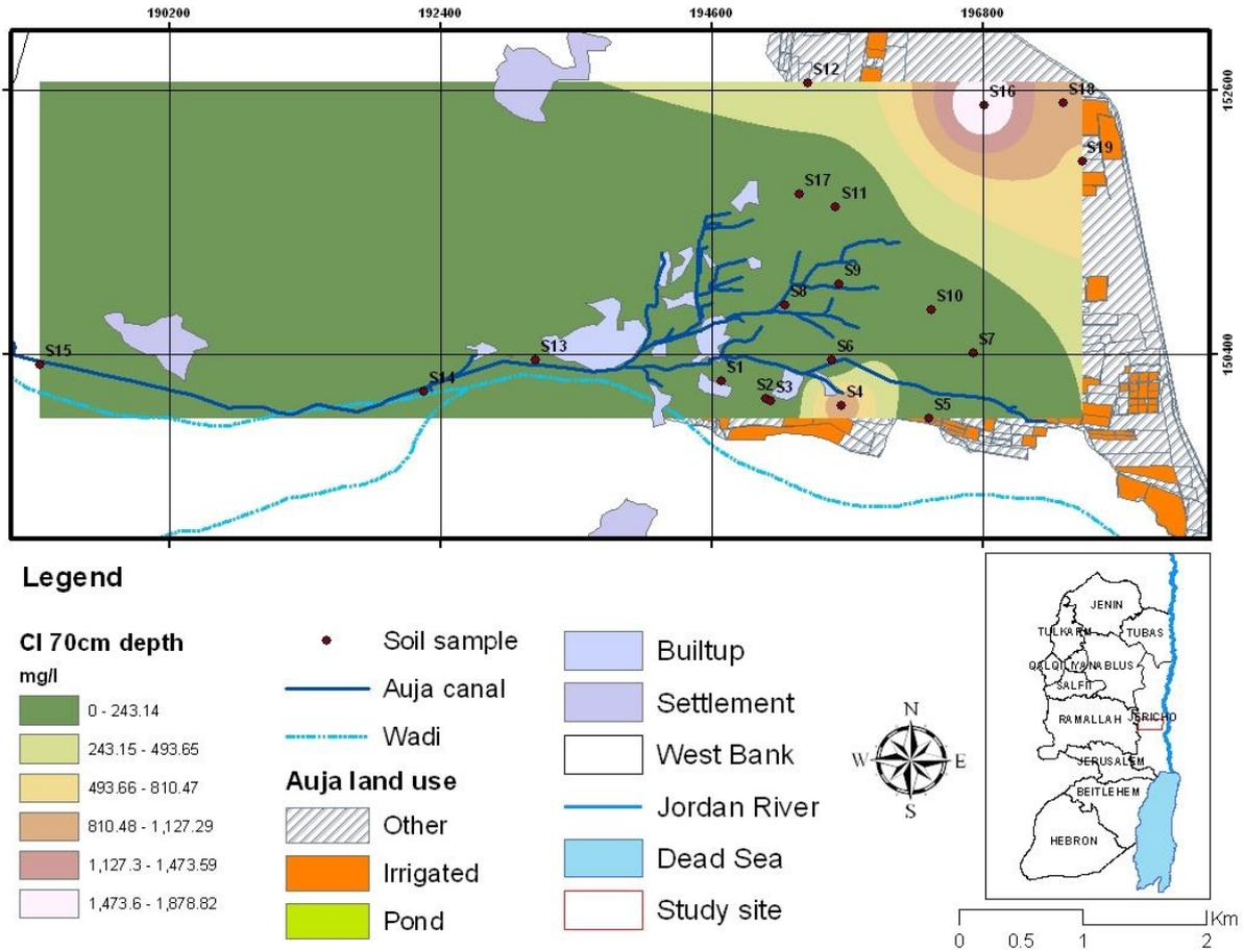
Figure10.22: Chloride concentration of (50-70 cm) depth at the CSA.
