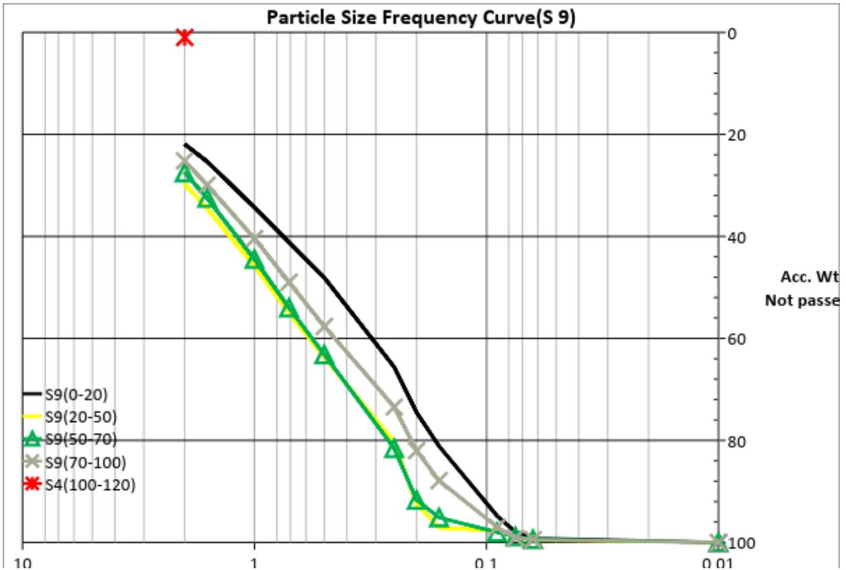
Figure 10.9: Particle size Frequency cure of Sample no.9, ( S9 )
