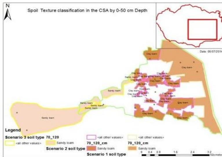
Figure 3.15c: Soil classification based on Soil Texture analysis in the CSA
