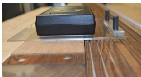
Fig. 3 Semi-automatic measuring device for exact positioning of the grain angle meter
