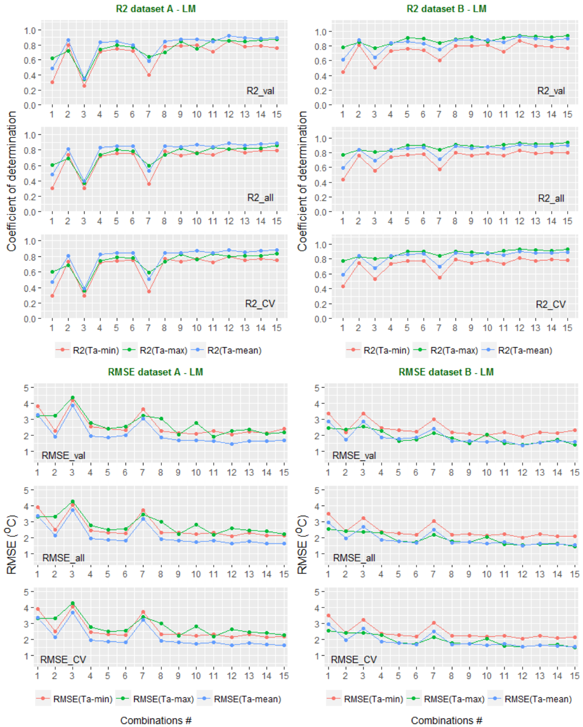
Figure 6.7. Comparison of accuracy ( R^2 and RMSE) when applying the LM algorithm to the validation dataset (_val), the full dataset (_all), and a cross-validation (_cv) of all combinations. The x-axis shows the combination number. The y-axis shows the values of RMSE ( ^{\circ}\text{C} ) and R^2 .
