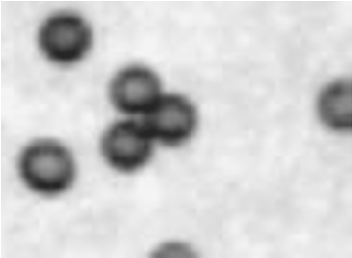
Figure 3.4: Charging and sticking of glass particles in a drop tower experiments (Image from private communication with Prof. Gerhard Wurm, Universität Duisburg Essen). URL: https://www.uni-due.de/imperia/md/images/physik/agw/sticking.gif .
