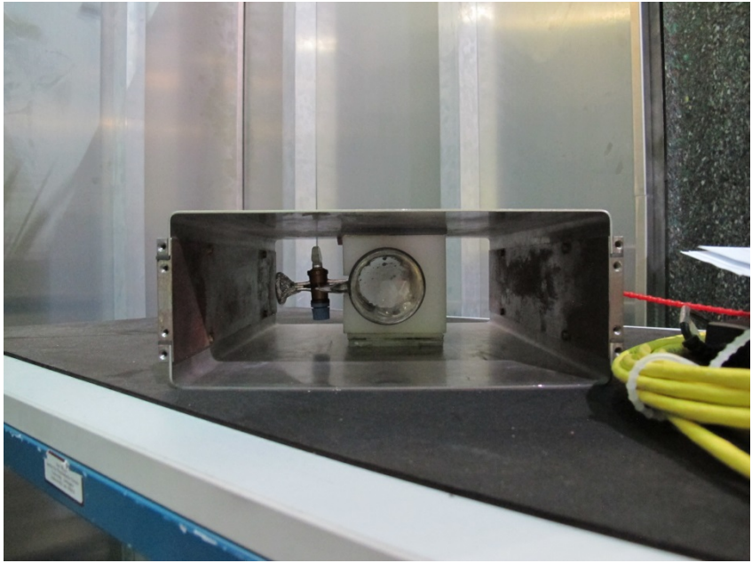
Fig. 10: ^3\text{He} -cell inside guide-field box. The box holds the cell in position and provides a homogeneous permanent magnetic field to preserve the spin polarization of the helium.
