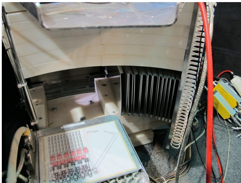
Fig. 6: A photo of the multi-detector with the eleven single detectors in parking position on the right side. The detector tubes are concealed by their guides.
