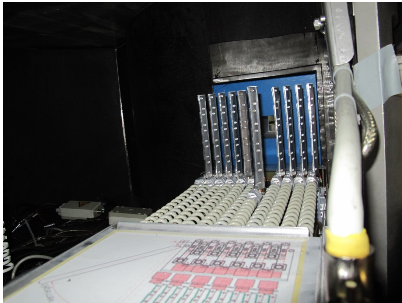
Fig. 5: Backside of multi-analyzer blades, viewing direction towards sample table
