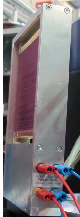
Fig. 28: Photo of flipper 2 shows the windings (differently colored wire for both coils) and power connections for both coils
