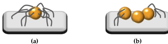
Figure 4.34: Illustration to demonstrate the formation of small and large assemblies. (a) A higher grafting density of star polystyrene can form a protective shell, thus smaller domains can be obtained. (b) A lower grafting density leads to larger domains, because of the aggregation of gold nanoparticles.
