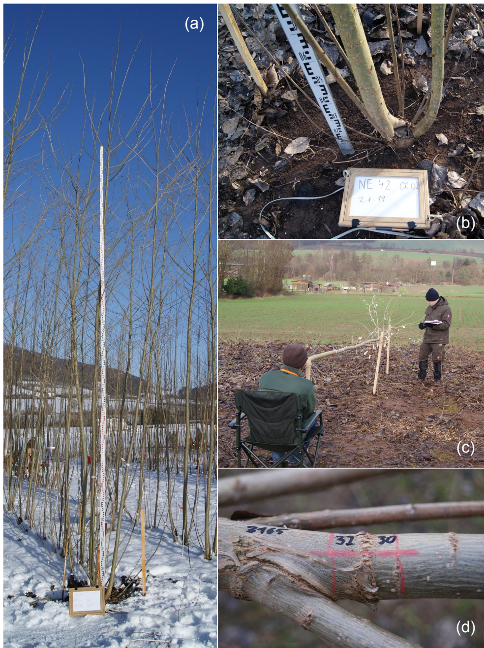
Figure 3.4: Exemplary display of some steps in manual measuring. Panel (a) shows a tree of the clone 'Max 1' photographed from the southern direction facing north. The trees in the plot margin have already been removed. Panel (b) contains a close up of the root stock of a 'Hybride 275' tree. The pole on the left marks the north direction. In panel (c) a cut off stem of one of the trees is fixed horizontally for measurement. Some of the labels that were applied to the GUs for identification are visible. Panel (d) shows further marks made directly on the stem for orientation. Shown is the scar left at the shoot base between a prolongation GU and its mother GU.
