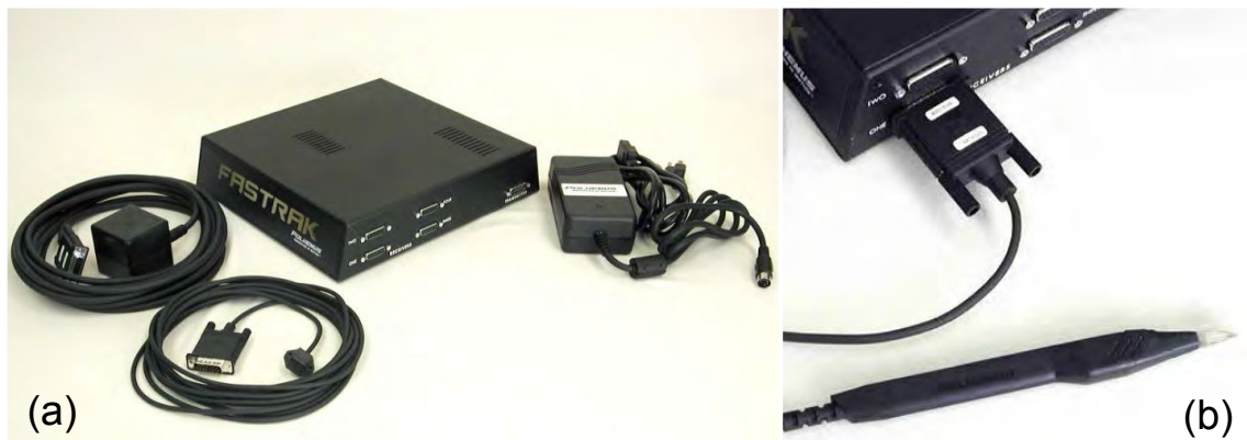
Figure 3.6: Components of the FASTRAK system. In panel (a) the System Electronics unit (SEU; middle), the transmitter (black cube, left), the standard receiver (bottom) and the power supply (right) are shown. In panel (b) the stylus is shown that also works as a receiver (Image source: Polhemus, 2012, (a) p. 1, (b) p. 25).
