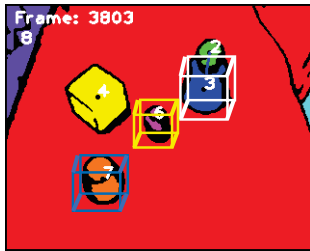
Fig. 5. Defining betweenness by AABBs. In this scene, yellow AABB is between white and blue AABBs.
