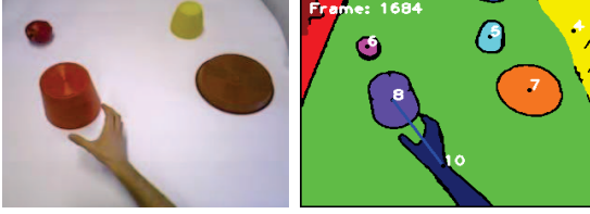
Fig. 2: A frame in MANIAC dataset (a) before and (b) after the scene segmentation. Segments are identified by different colors and segment numbers.
